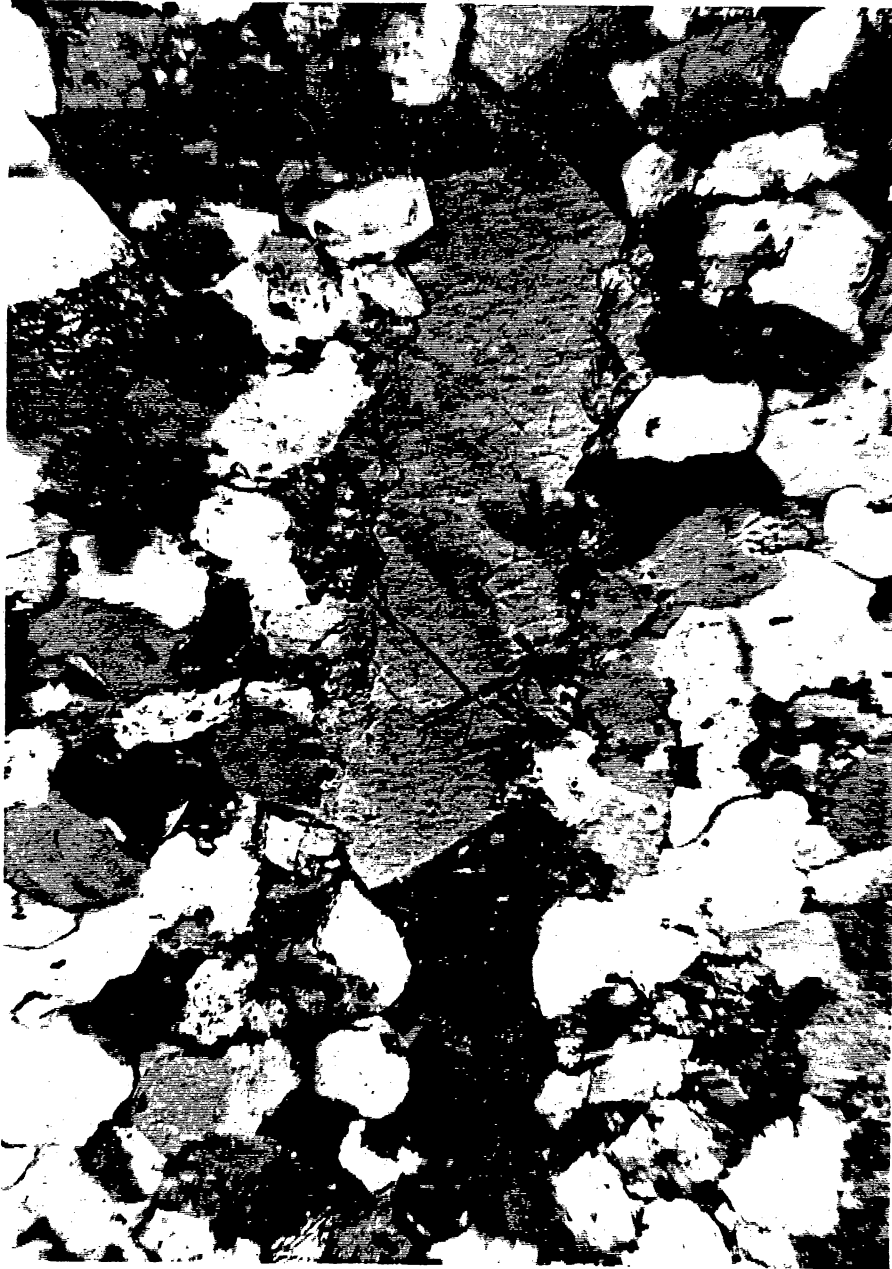
Figure 48. Photomicrograph showing superposition of infilling mineral phases in Travis Peak fracture. Sample is from Holditch SFE No. 2 well.
