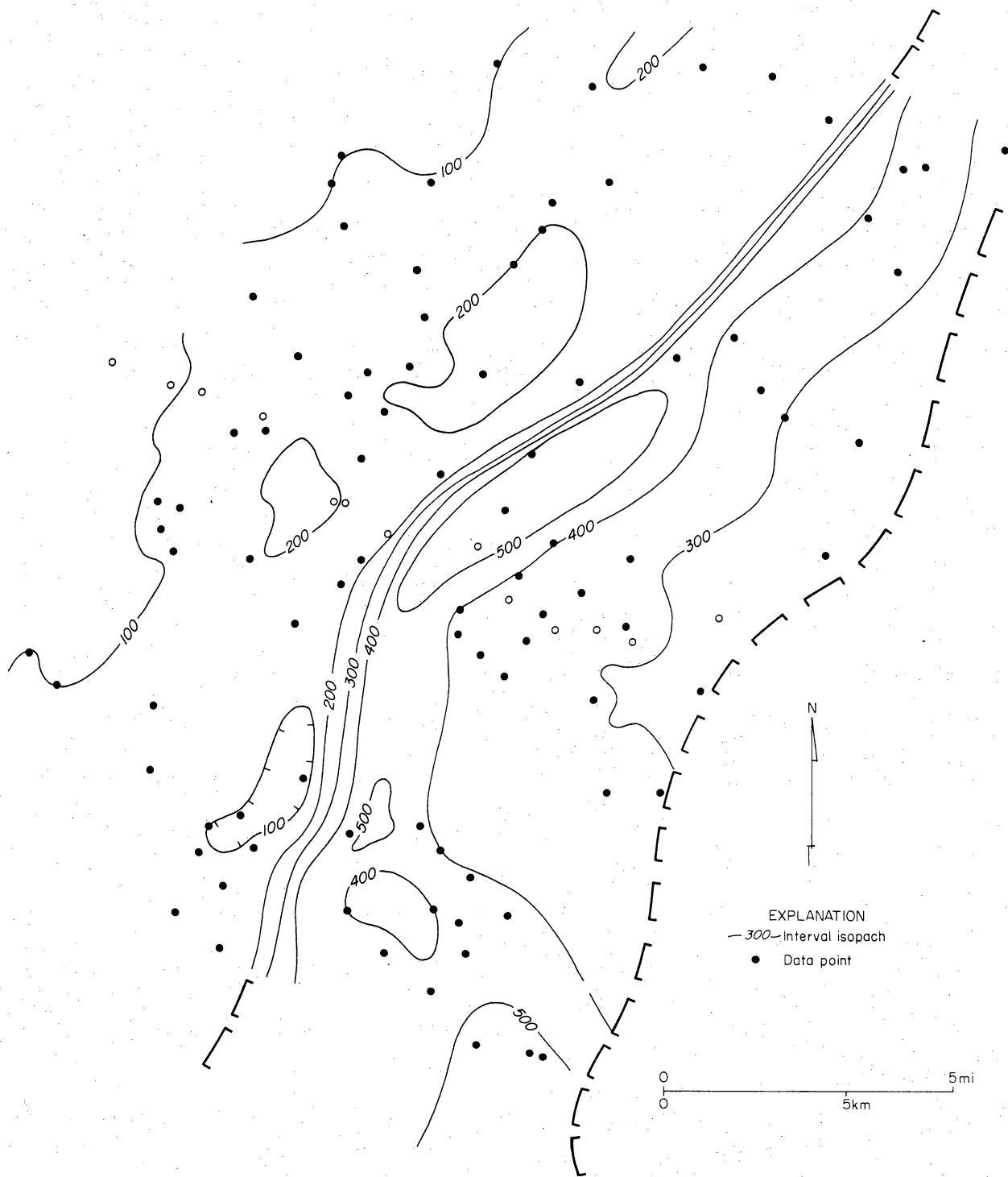
Figure 8. Interval isopach of the upper map unit. Again, note thickening across the central growth fault.
