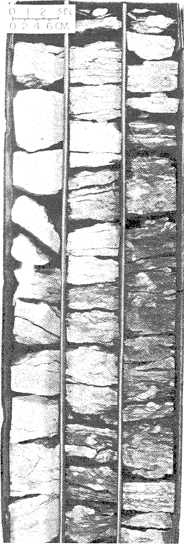
Figure 16. Core photograph showing typical features of muddy siltstone to sandy siltstone (top of core) of the shelf facies.
