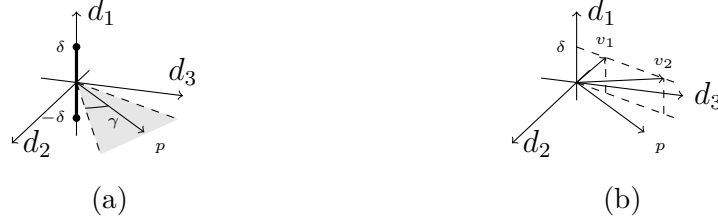
Figure 4.4: Possible cases for Algorithm 9. (a) The uncertainty sets for the unknown direction, d_1 , and the known directions, d_2 and d_3 . (b) Two possible cases for the gradient estimation in Algorithm 9.
