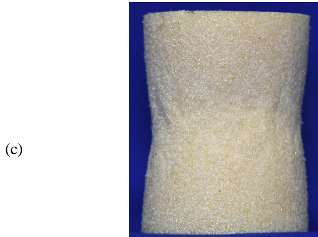
Figure 4.8: Results from a pure pressure experiment: (a) Expanded pressure-axial shortening response at the onset of lateral crushing. (b) Photographic images showing the specimen as it crushes. (c) Postmortem image of a test specimen crushed by external pressure.
