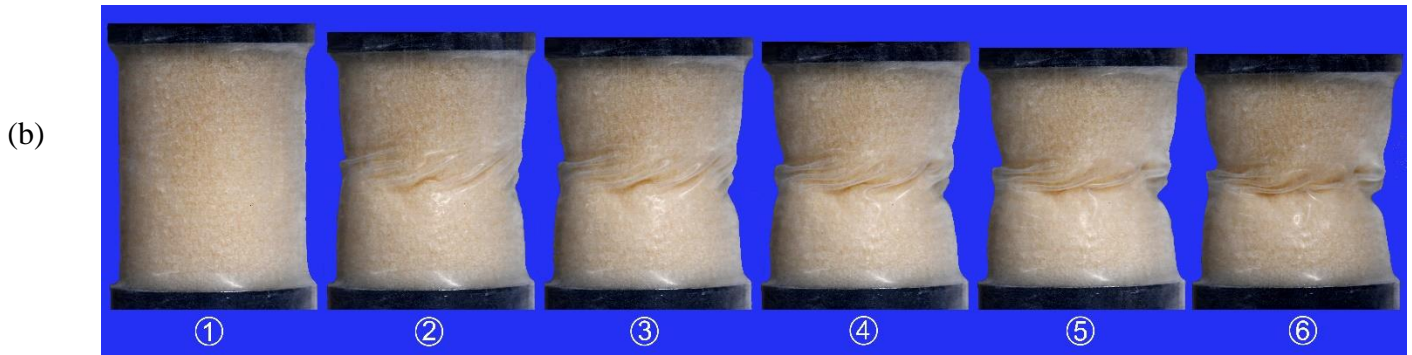
Figure 4.7: Summary of results of specimen FM8 compressed under 8.12 bar external pressure. (a) Axial stress-shortening response. (b) Sequence of photographic images showing the evolution of localization; correspond to numbered sites on the response in (a).
