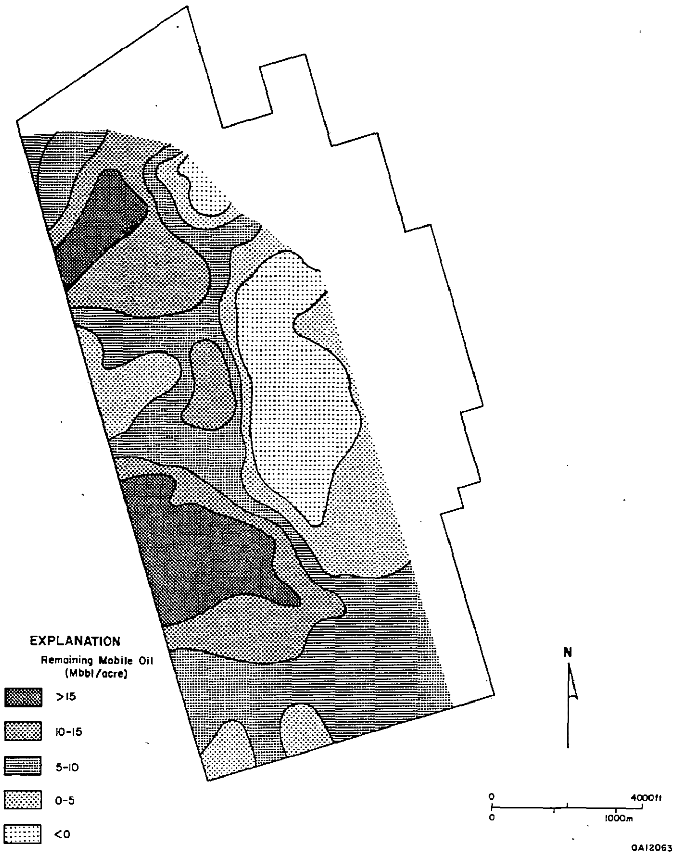
Figure 33. Remaining mobile oil map calculated using R_w values obtained from analyses of produced water.
