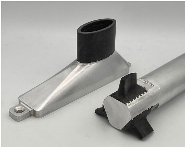
Figure 10. Multi-material parts with aluminum and composite regions joined using mechanical interlocking.
