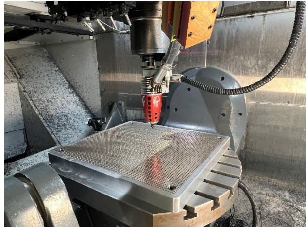
Figure 1. Mechanically interlocking print bed in a HAAS Machining Center.
