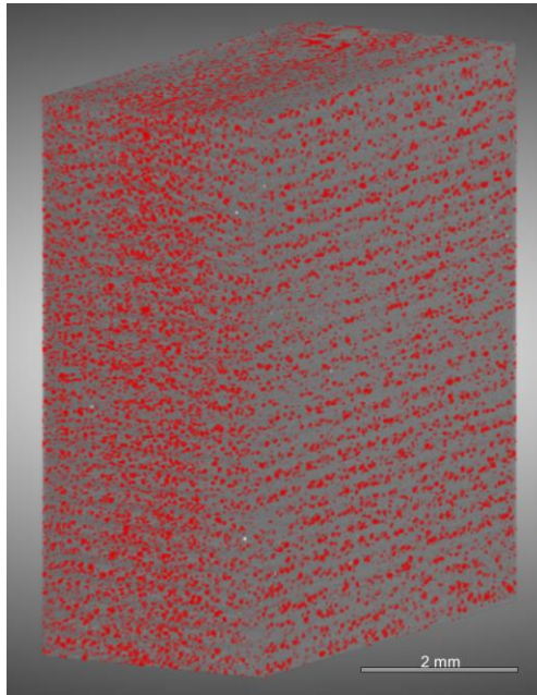
Figure 6: Annealed sample with \mu CT void reconstruction.
