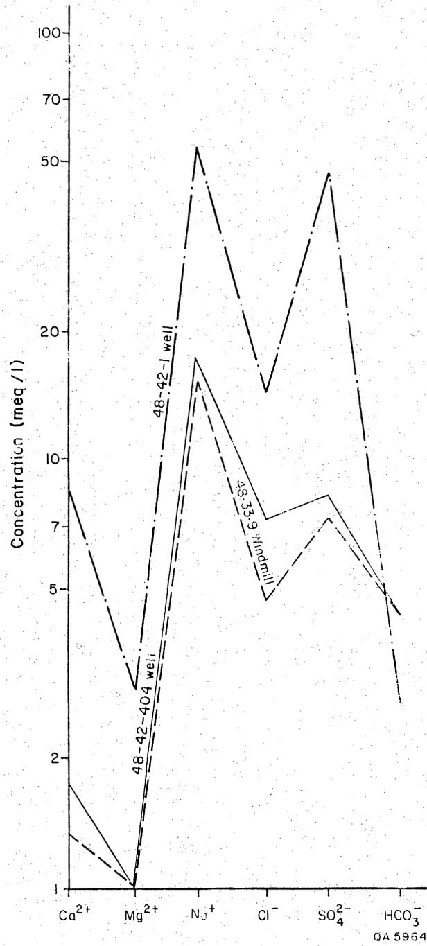
Figure 39. Salinity diagram of ground-water samples of the bolson-fill aquifer in the S-34 study area. Well location is shown in figure 32.
