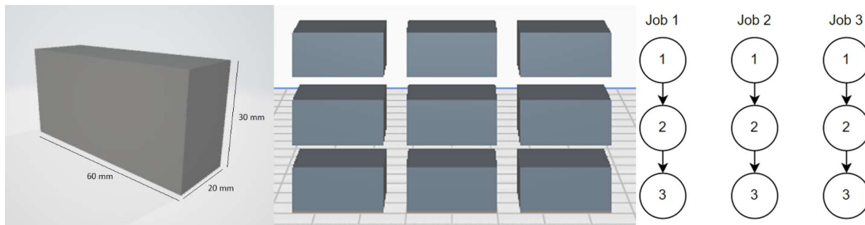
Figure 5: Small Box Test Case. (a) Full Model, (b) Chunked Model, (c) Dependency Tree
