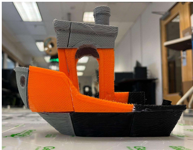
Figure 13: Assembled Model of 3DBenchy Test Case (Orange: Printer 1, Black: Printer 2, Gray: Printer 3)
