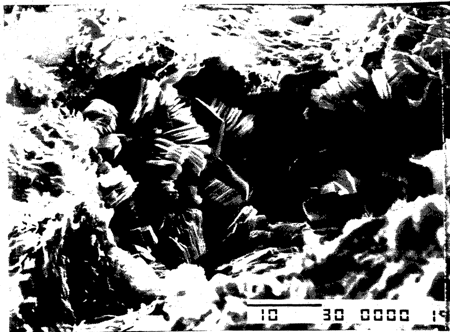
Figure 14. Authigenic kaolinite within a secondary pore. Sample from a depth of 6,985.5 ft in the Mobil Tip Top No. T71X-6G-28N-113W well. SEM photo by K. L. Herrington. Scale bar is 10 \mu\text{m} .
