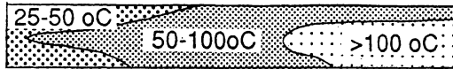
FIGURE 12. Cross section of temperature distribution after injection of 2.1 pore volumes of hot water. After Dietz (1972).
