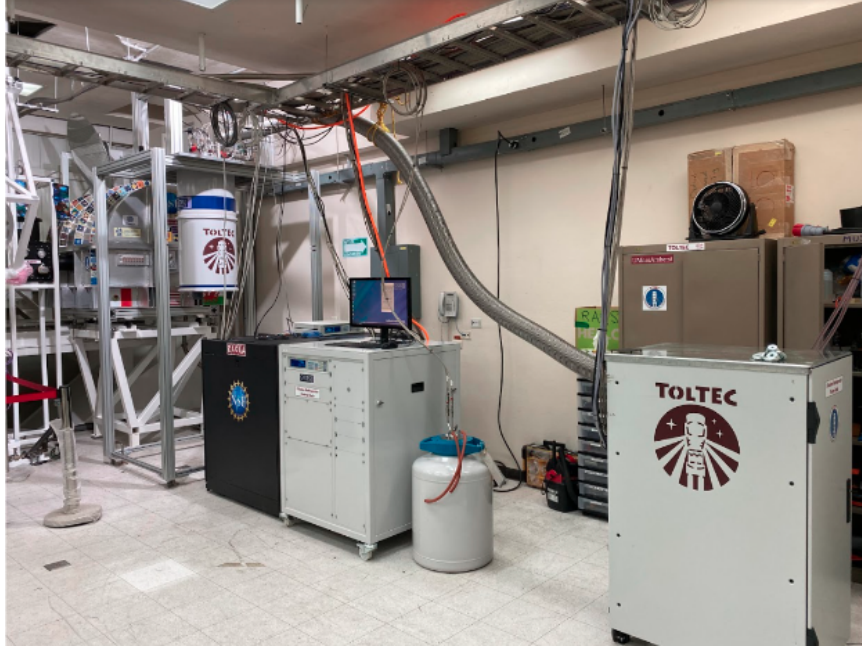
Figure 4.1: A photo of the TolTEC camera inside the receiver cabin at the Large Millimeter Telescope (LMT). In the foreground are the pumps, cold trap, and electronics rack for TolTEC’s dilution refrigerator; in the background is the instrument itself facing the warm coupling optics (see Fig. 4.3). TolTEC was installed in the LMT receiver cabin in December 2021.
