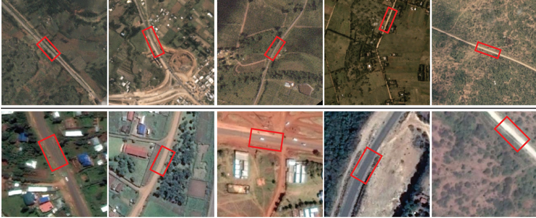
Figure 5.5: A Series of roads from two data sources; Planet Labs(top) at 3m/pixel and Google Earth Pro (bottom) at \sim 1.6\text{m/pixel} . The different sizes, visibility and resolutions of the road images highlight the heterogeneity of our dataset. The red rectangle indicates the range of the road segment over which the IRI measurements are averaged.
