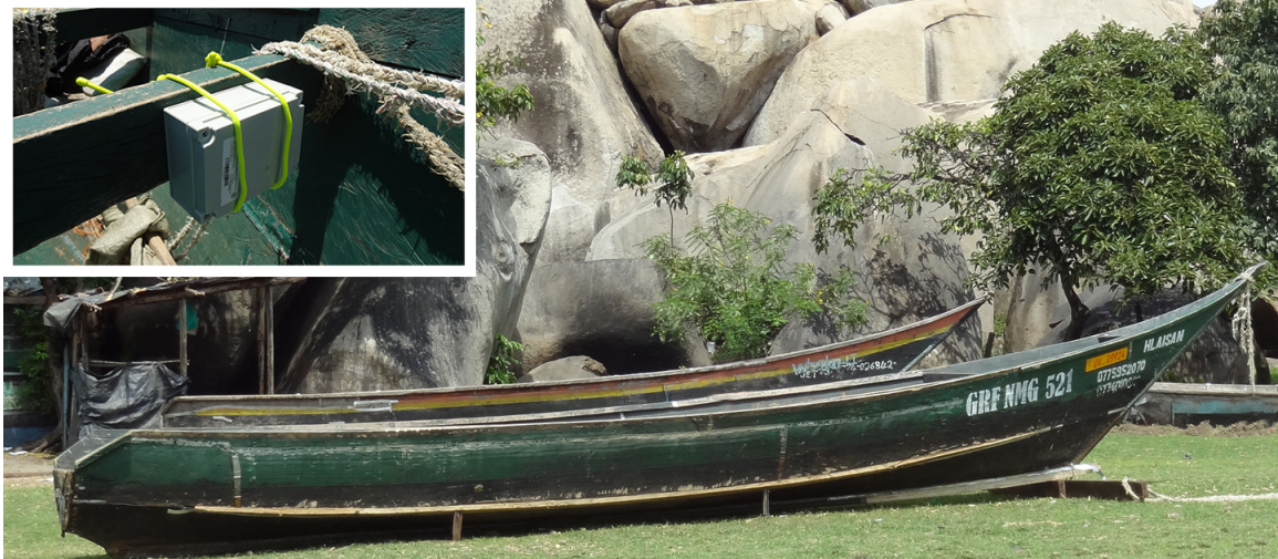
Figure 6.1: Example fishing boat on Lolwe Island. Inset: boat tracking device attached to the boat before deployment.
