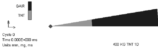
Fig. 4. Mesh used for the generation of the explosion (400 kg TNT).
