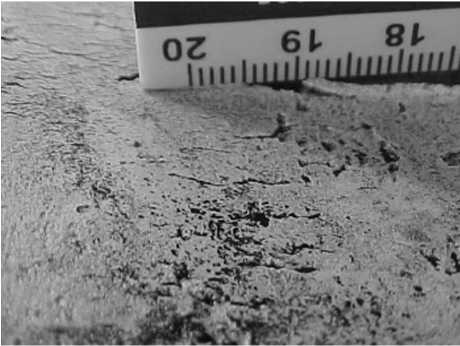
Fig. 6. Secondary cracks found by magnetic particle inspection in failure case 3 ( \times 3 ).
