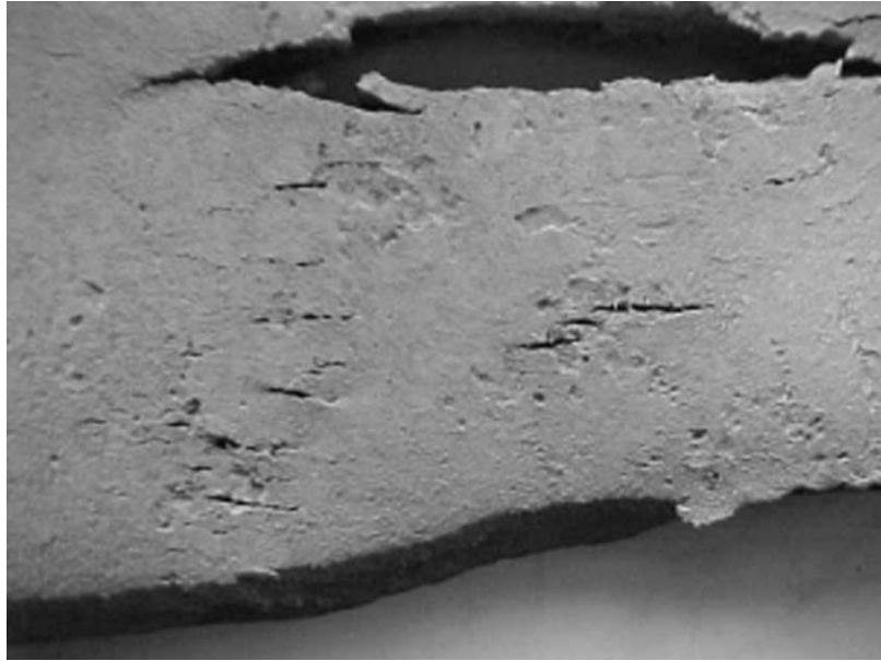
Fig. 4. Secondary cracks found by magnetic particle inspection in failure case 2.
