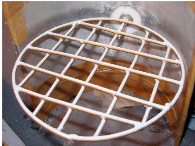
Figure 2. Picture of the rimed target. The wires of the network are 2 mm in diameter.
