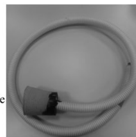
3 Corrosion sensor developed at CNEA: different components of sensor (left); sensor conditioned and ready for installation in HST-2 test (right)
