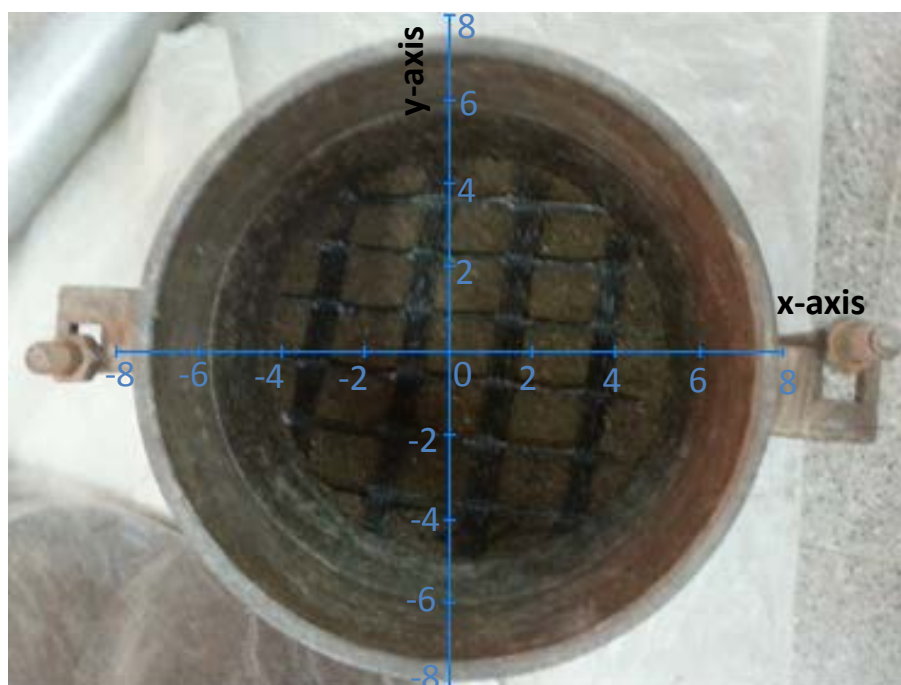
Figure 7: Axes (Unit: cm) used to measure the vertical displacements in the geogrid.
