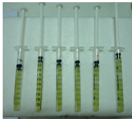
Figure 13. Photography of syringes containing dispersions of ionic complex NIPA:AAc (70:30)-OFL (50% neutralized acid groups) prepared so until 1% dispersion of OFL.
