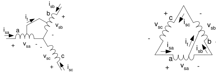
(a) Short circuit between turns in phase a and b in a \mathbf{Y} -connected stator.
