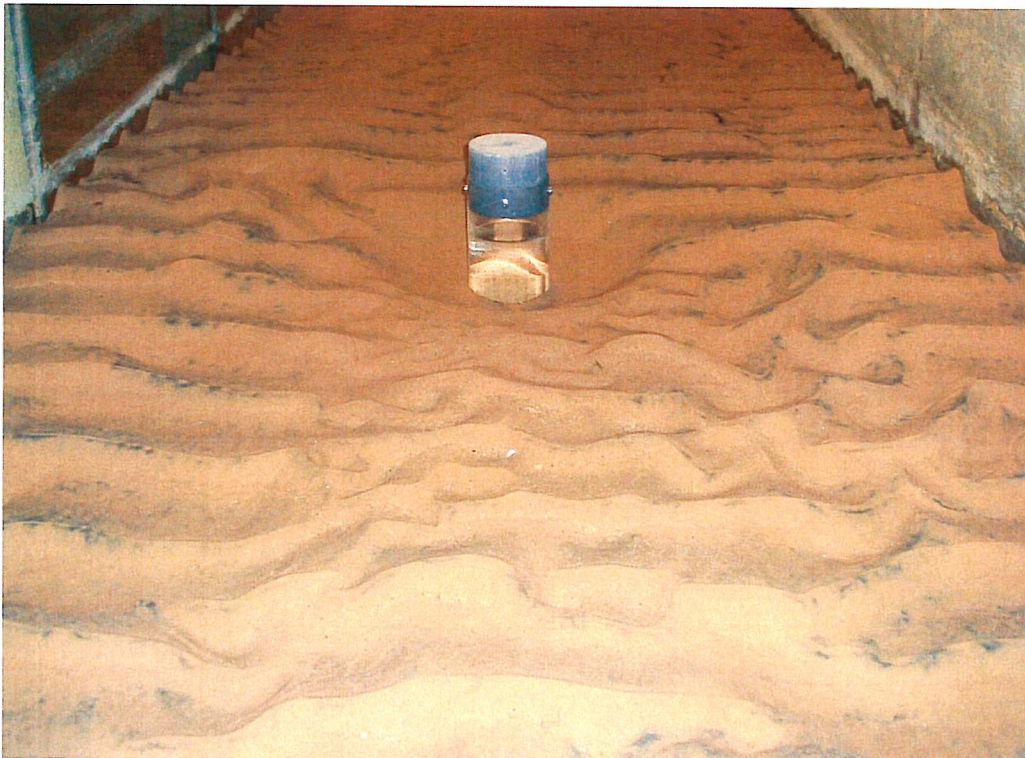
Figure 15. The picture is from test 1.5. In test 1.5 and 1.6 there was both ripples and a small scour hole.
