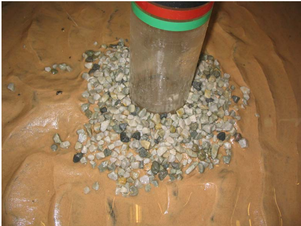
Figure 1.33. Shape of scour protection at the end of 3.4. No severe damage.
