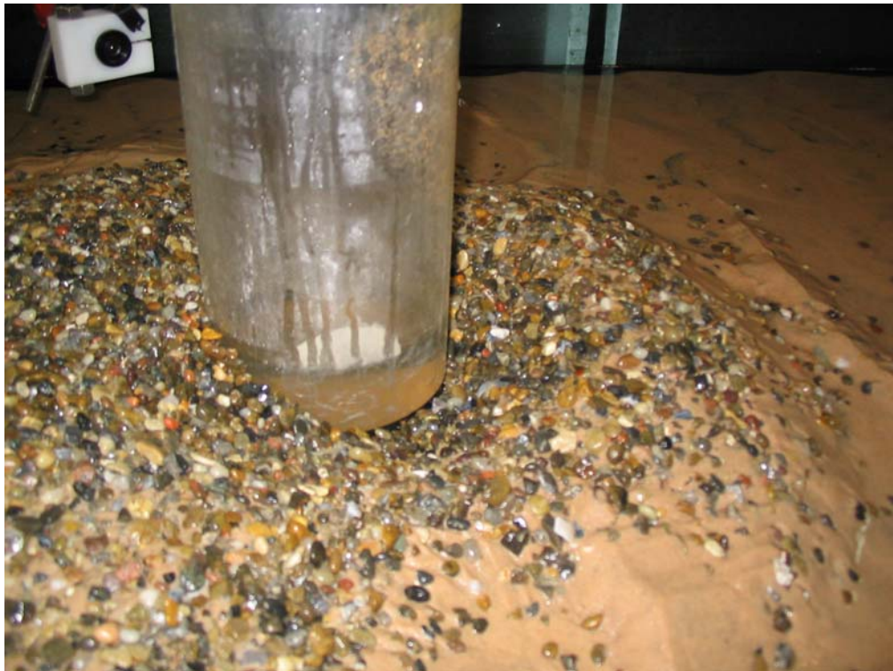
Figure 1.29. Shape of scour protection at the end of 3.2. Some damage. 1.5 m scour depth.
