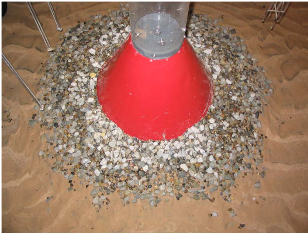
Figure 1.53. Shape of scour protection at the end of 3.14. No damage occurred.
