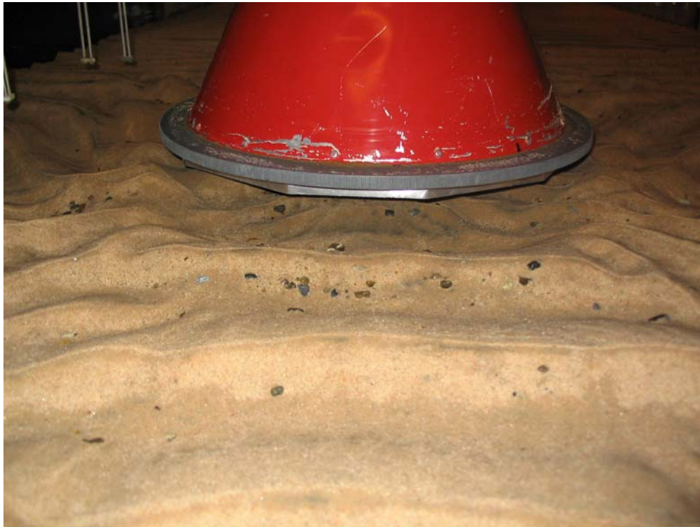
Figure 1.7. Scour hole at the end of 1.7.
