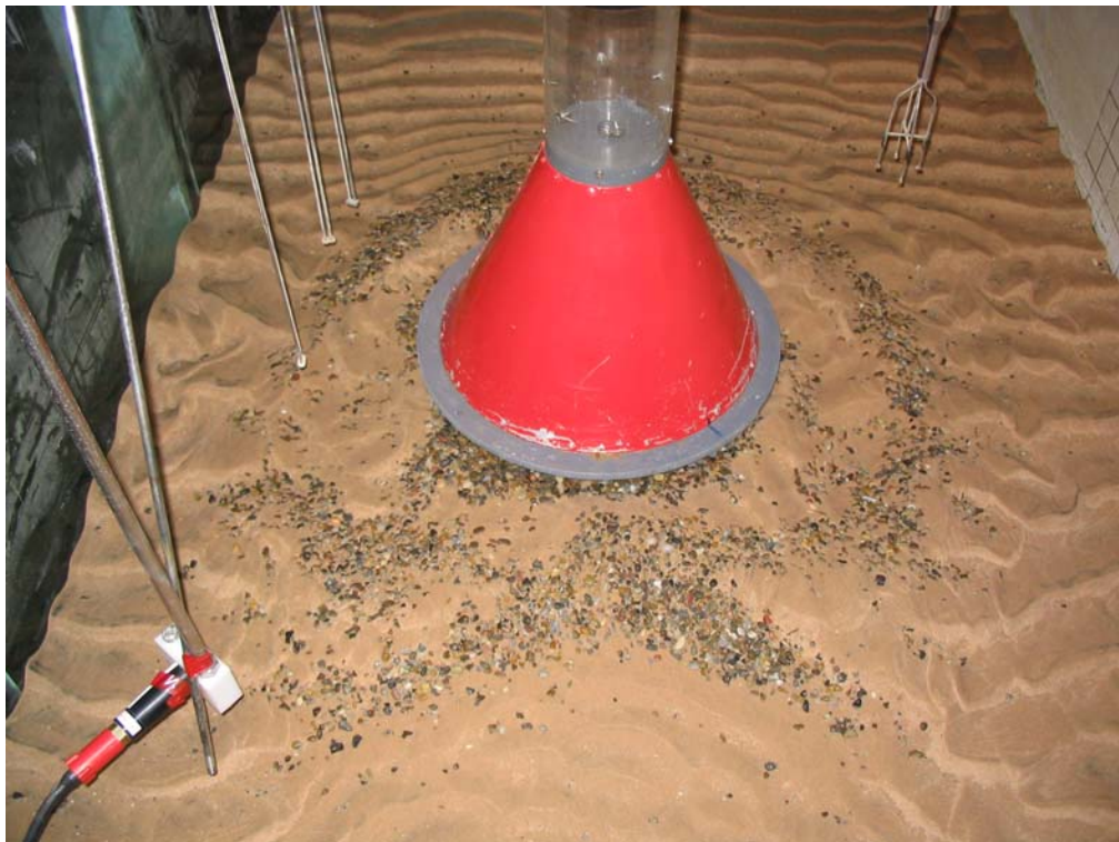
Figure 1.47. Shape of scour protection at the end of 3.11. Complete damage. 1.0 m scour depth.
