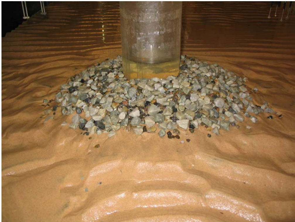
Figure 1.39. Shape of scour protection at the end of 3.7. No damage occurred.
