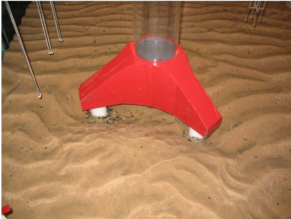
Figure 1.6. Scour hole at the end of 1.6. The scour is occurring underneath the structure.
