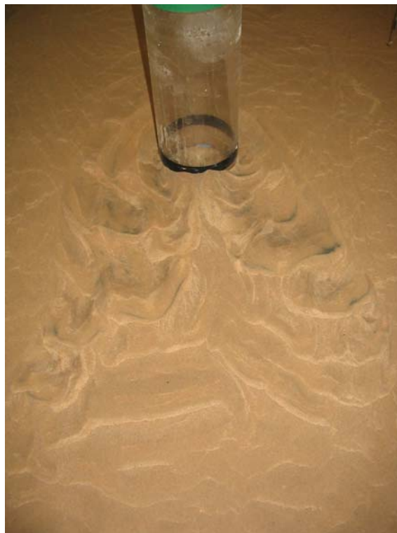
Figure 1.1. Scour hole at the end of 1.1.
