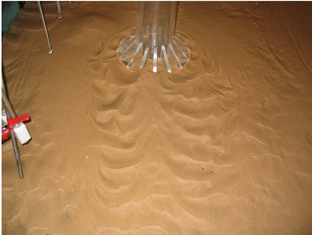
Figure 1.4. Scour hole at the end of 1.4.
