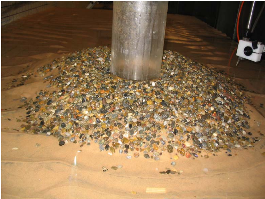
Figure 1.45. Shape of scour protection at the end of 3.10. No severe damage.
