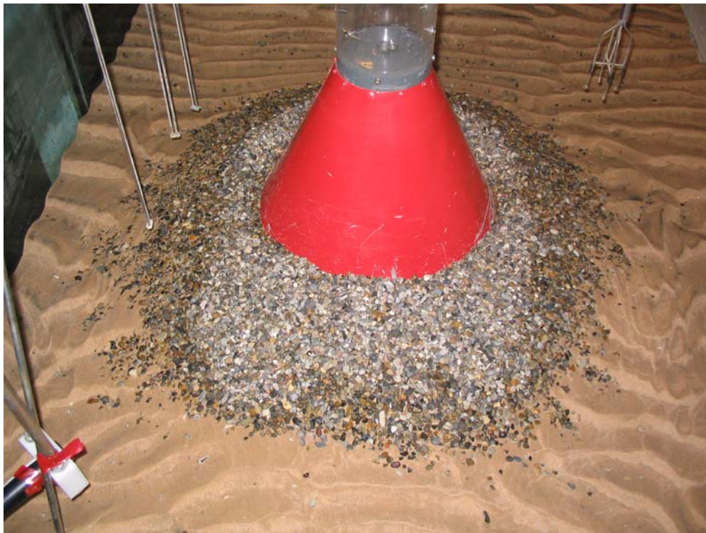
Figure 1.61. Shape of scour protection at the end of 3.18. No damage occurred.
