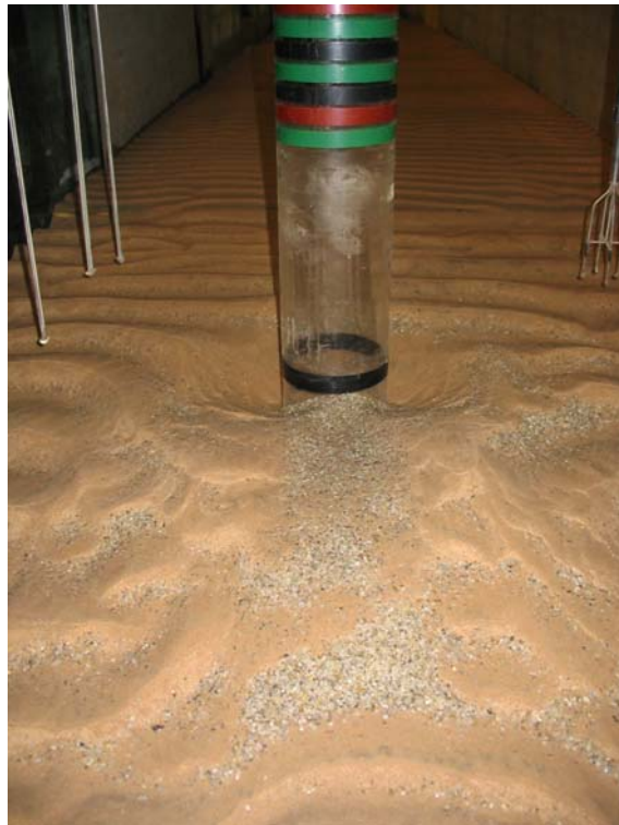
Figure 1.11. Shape of scour protection at the end of 2.2. Complete damage. 2.5 m scour depth.
