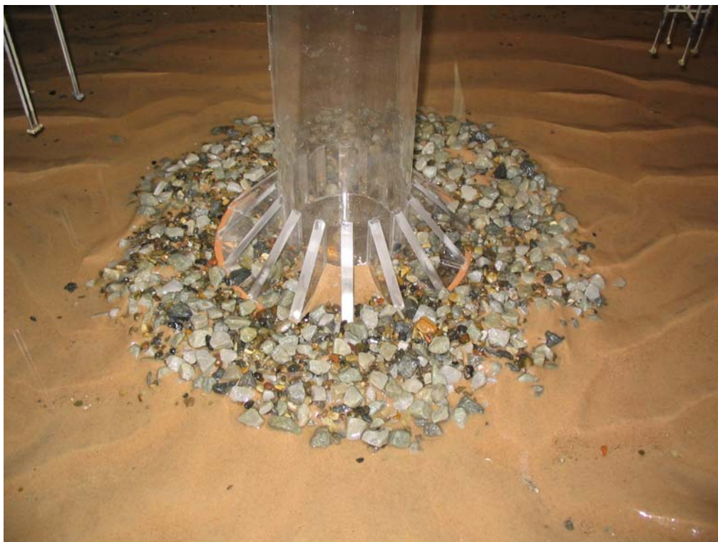
Figure 1.25. Shape of scour protection at the end of 2.9. No severe damage.
