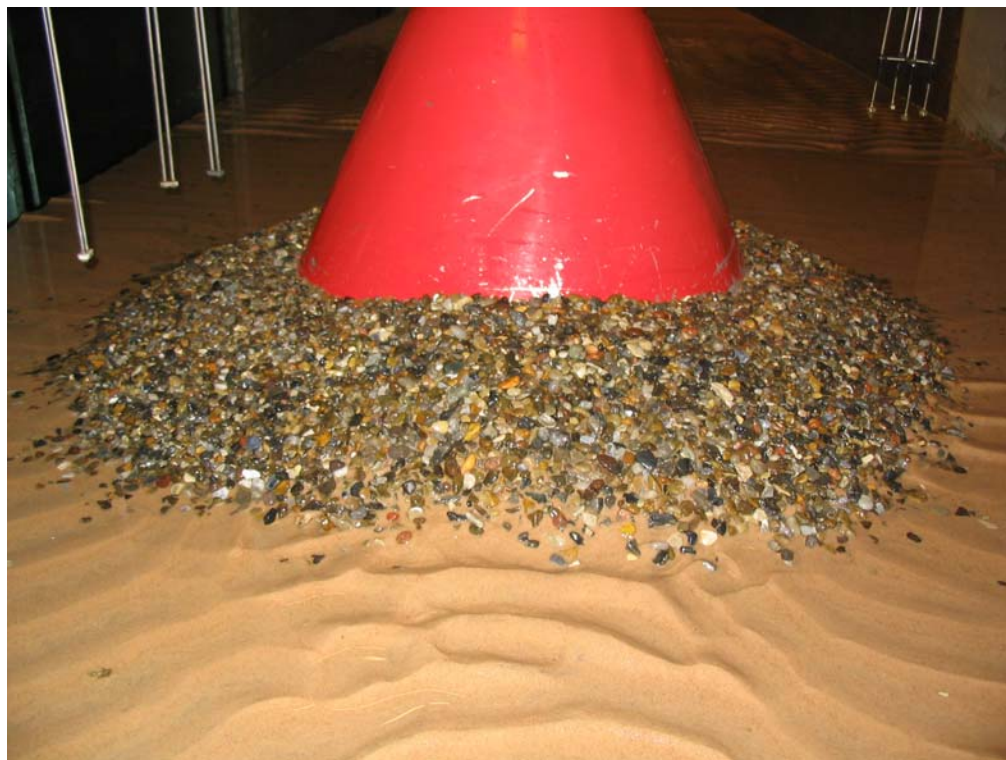
Figure 1.59. Shape of scour protection at the end of 3.17. No damage occurred.
