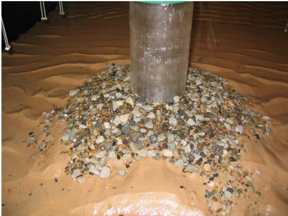
Figure 1.41. Shape of scour protection at the end of 3.8. No severe damage.
