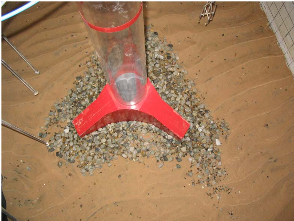
Figure 1.21. Shape of scour protection at the end of 2.7. No severe damage.
