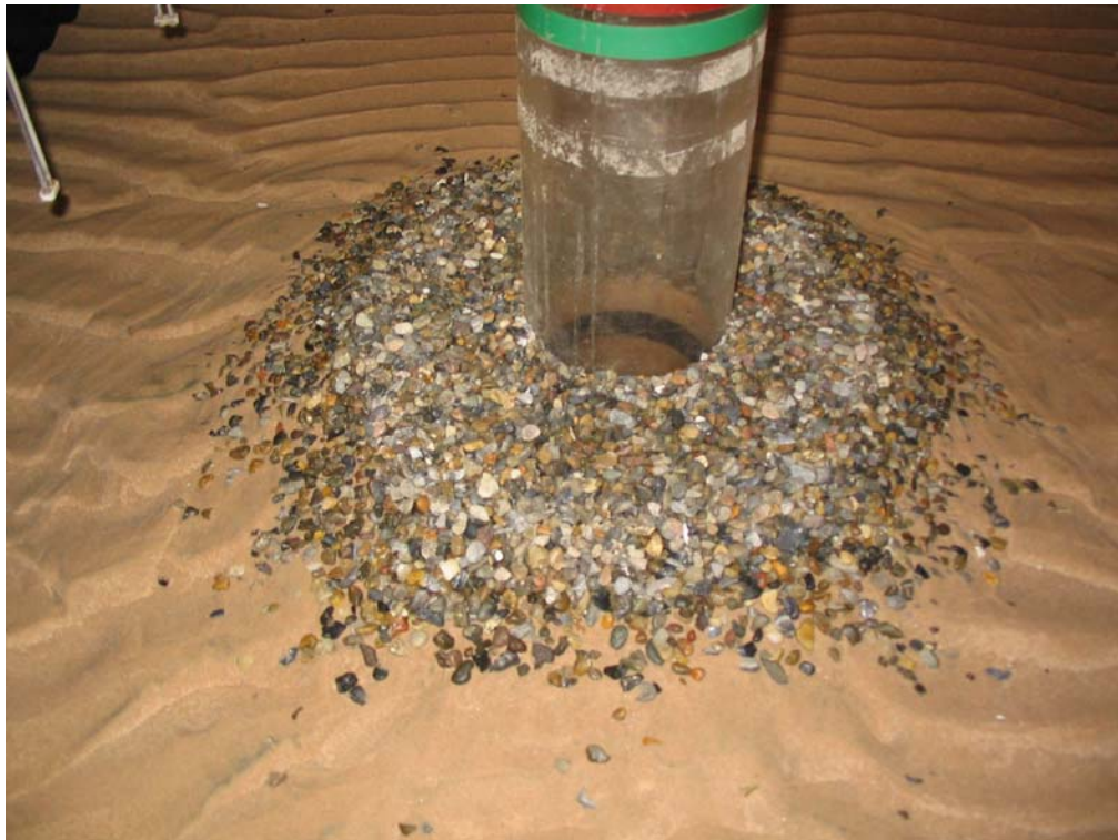
Figure 1.43. Shape of scour protection at the end of 3.9. No damage occurred.
