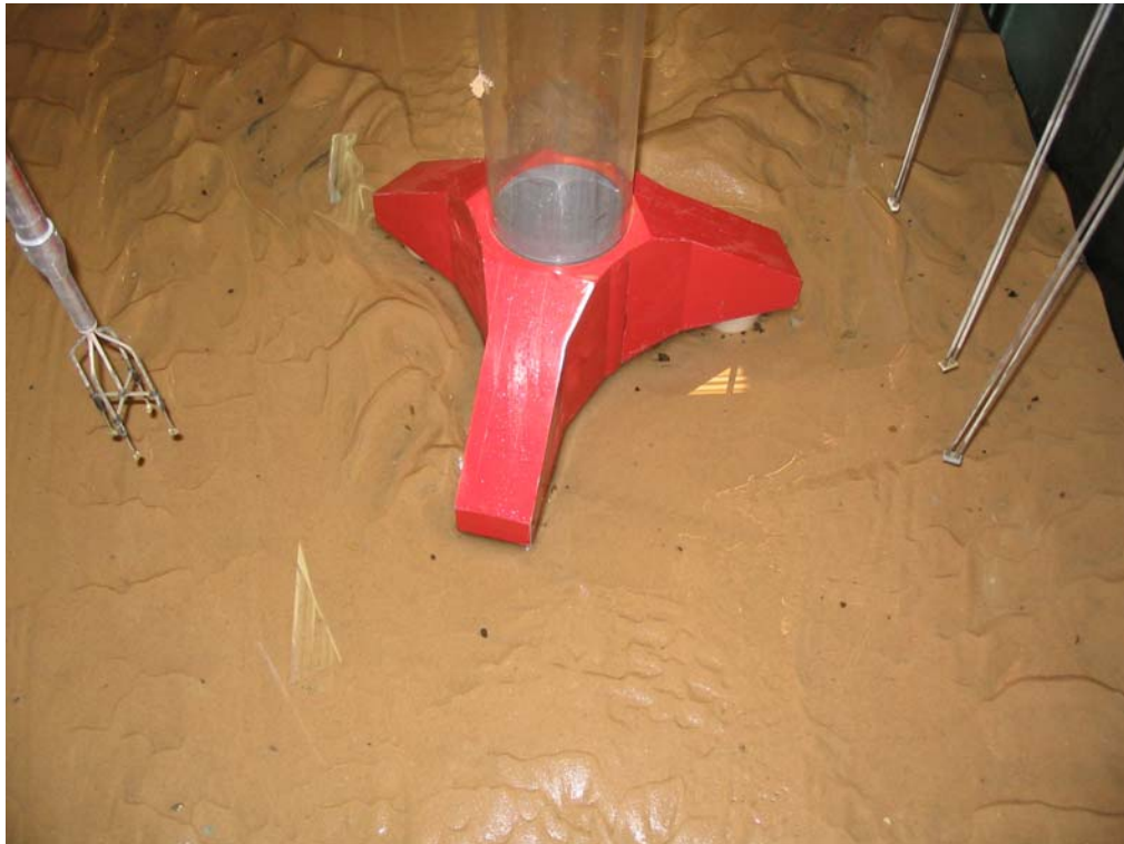
Figure 1.2. Scour hole at the end of 1.2. The scour is occurring underneath the structure.
