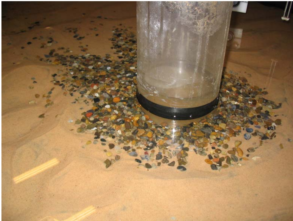
Figure 1.17. Shape of scour protection at the end of 2.5. Severe damage. 1.5 m scour depth.
