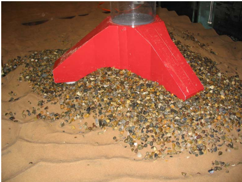
Figure 1.63. Shape of scour protection at the end of 3.19. Some damage occurred.
