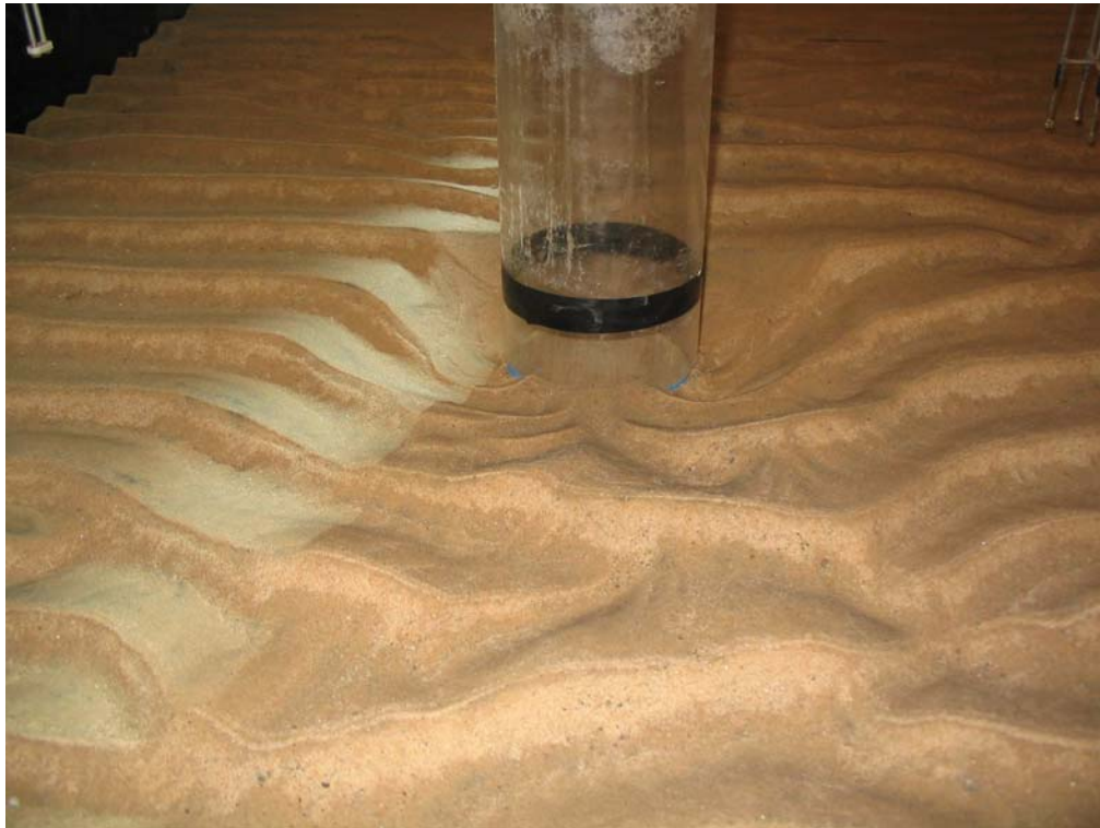
Figure 1.5. Scour hole at the end of 1.5.
