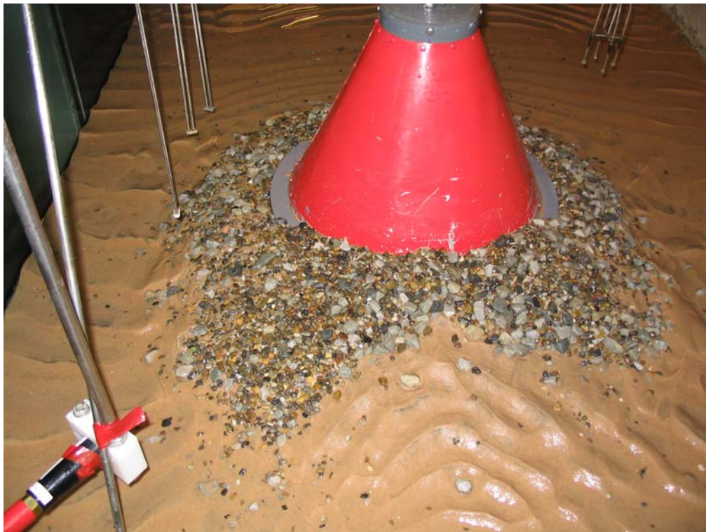
Figure 1.57. Shape of scour protection at the end of 3.16. No damage occurred.
