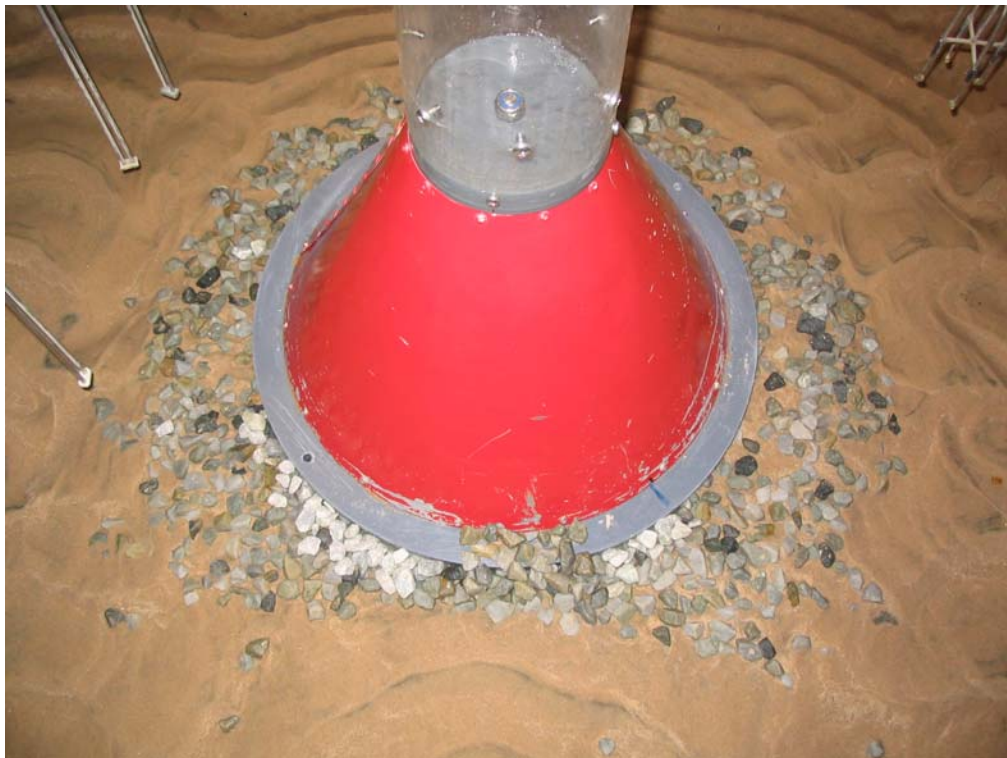
Figure 1.51. Shape of scour protection at the end of 3.13. Some damage. 1.0 m scour depth.
