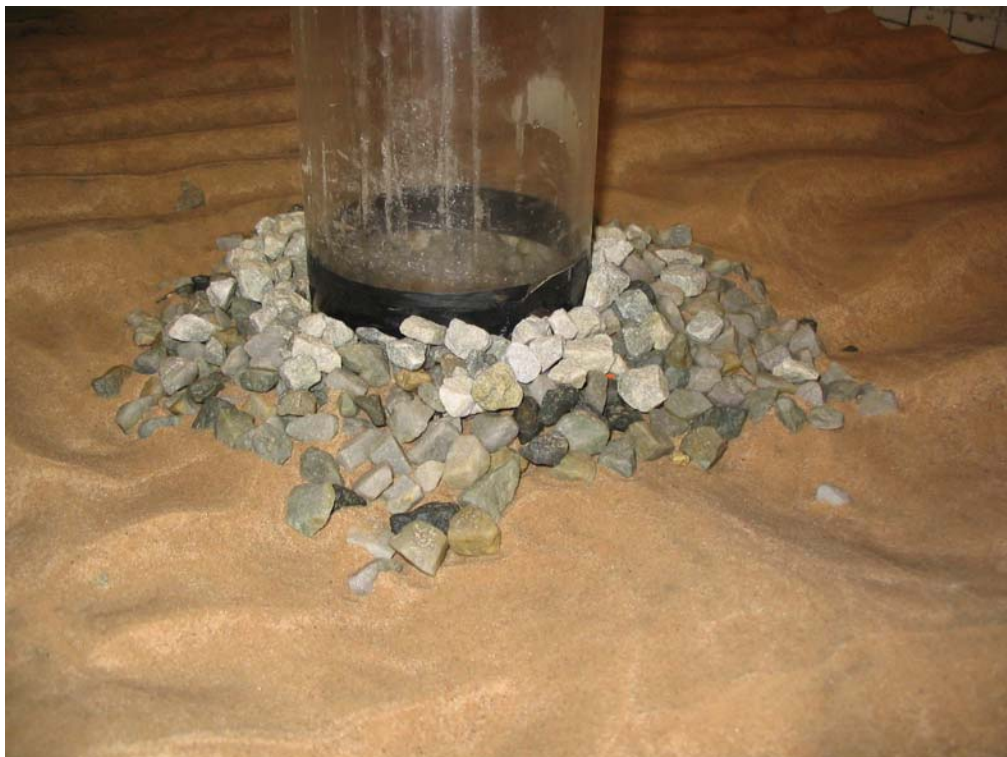
Figure 1.19. Shape of scour protection at the end of 2.6. No damage occurred.
