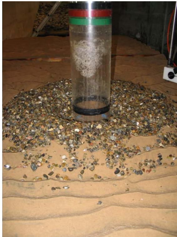
Figure 1.13. Shape of scour protection at the end of 2.3. Severe damage. 1.5 m scour depth.
