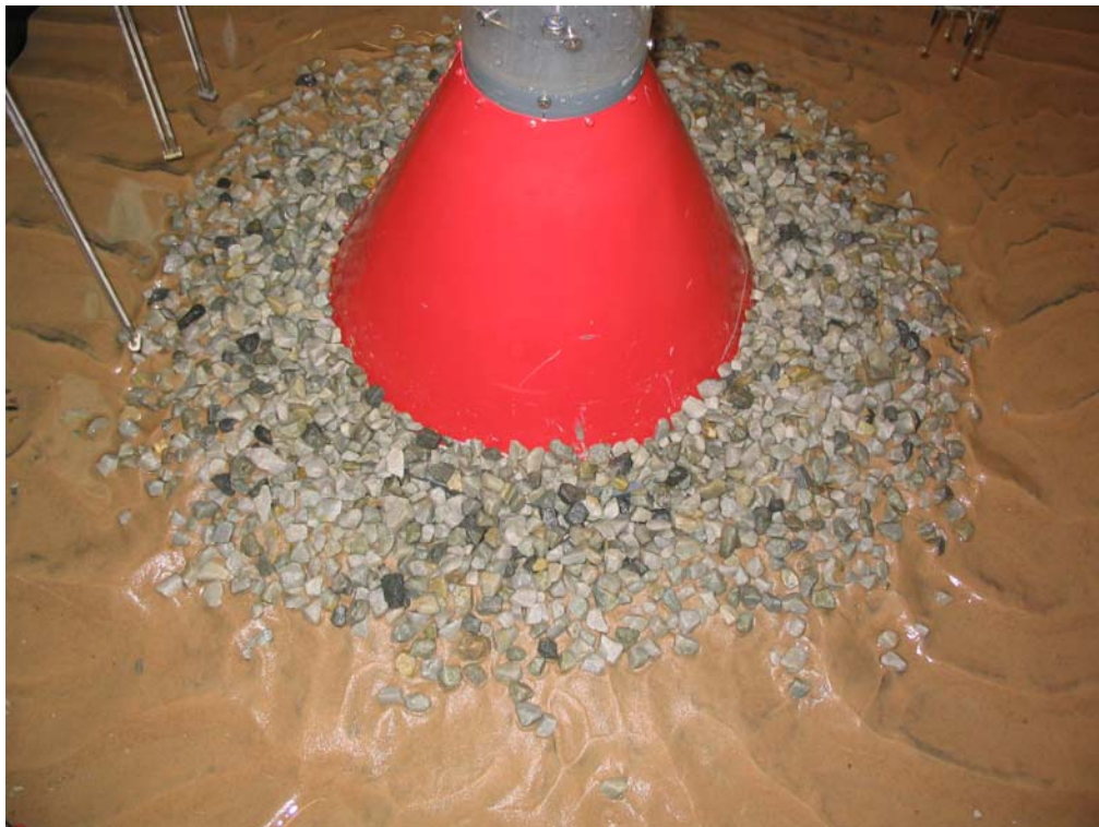
Figure 1.49. Shape of scour protection at the end of 3.12. No damage occurred.
