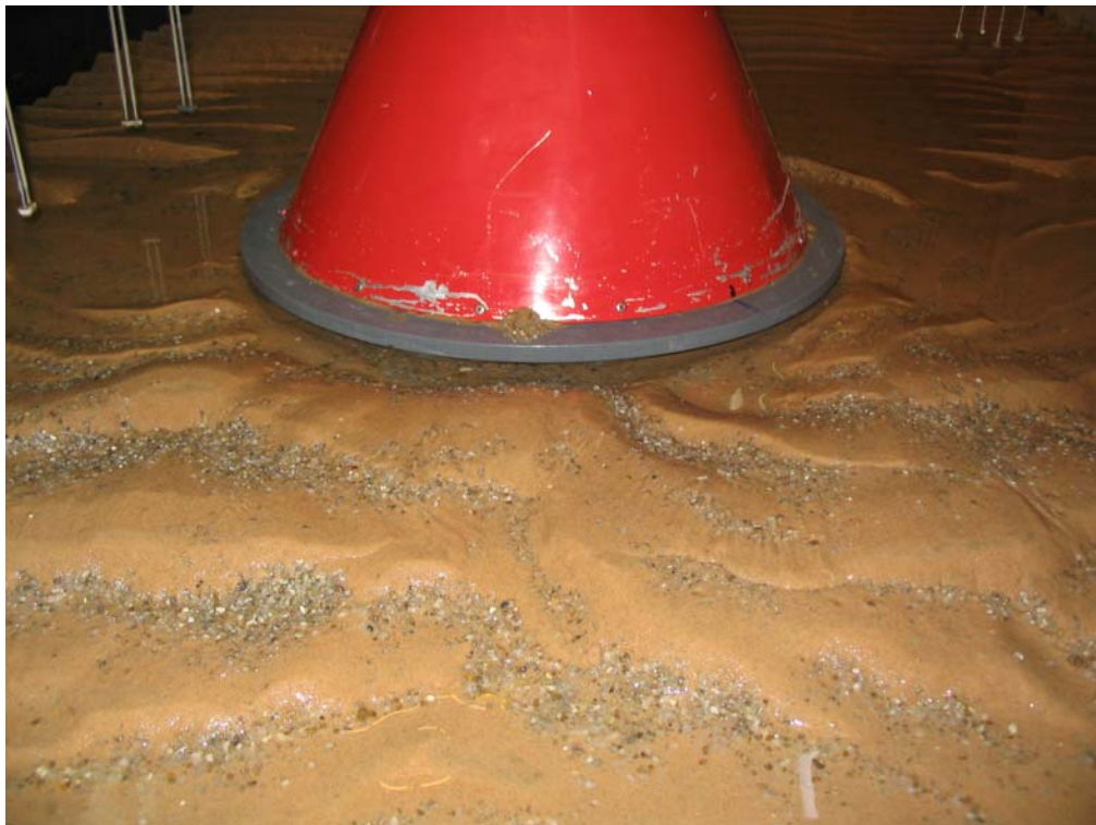
Figure 1.23. Shape of scour protection at the end of 2.8. Complete damage. 1.0 m scour depth.
