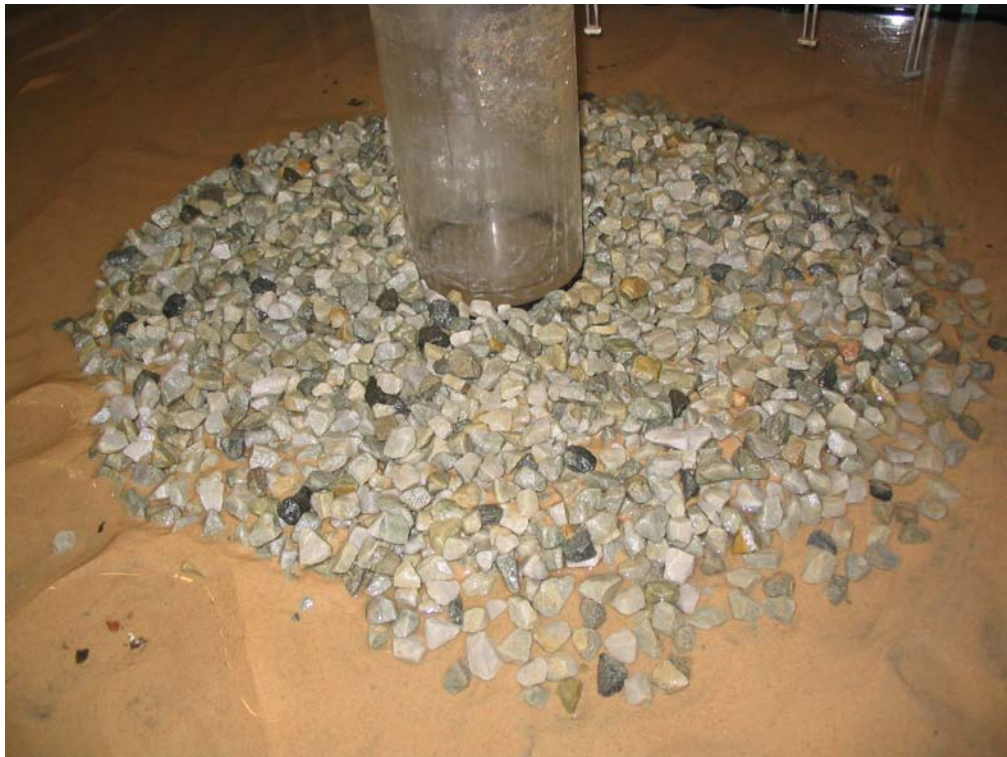
Figure 1.15. Shape of scour protection at the end of 2.4. No damage occurred.
