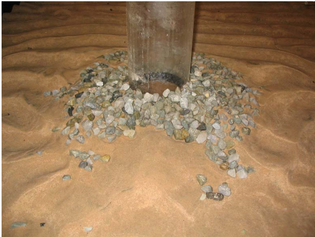
Figure 1.37. Shape of scour protection at the end of 3.6. No severe damage.
