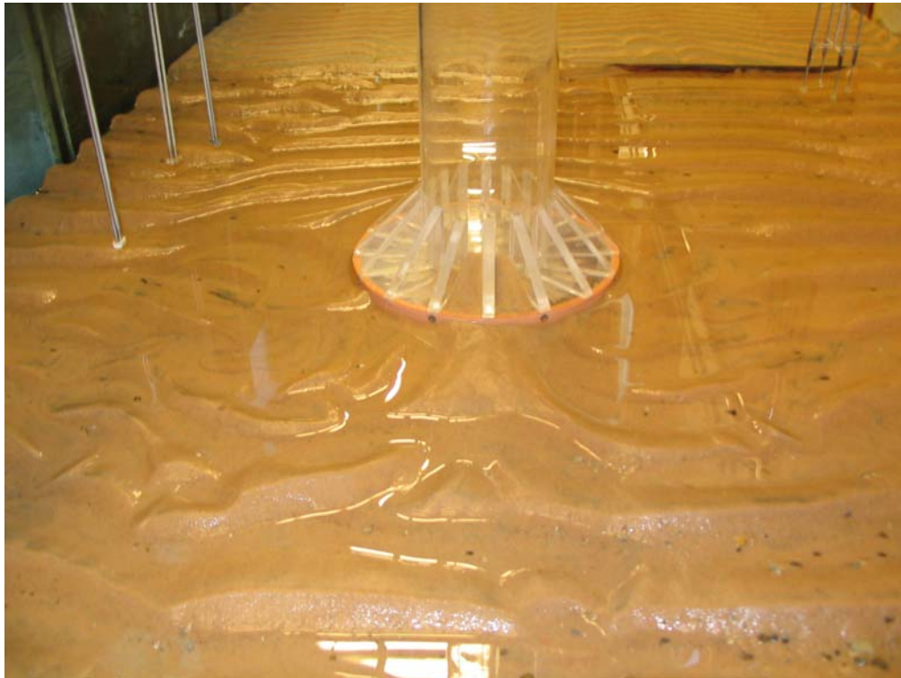
Figure 1.8. Scour hole at the end of 1.8.
