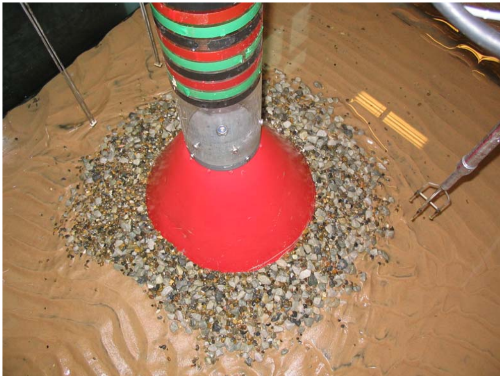
Figure 1.55. Shape of scour protection at the end of 3.15. No damage occurred.
