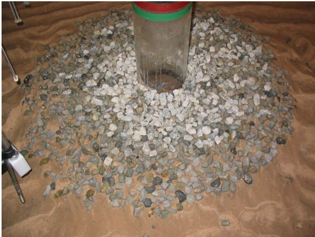
Figure 1.31. Shape of scour protection at the end of 3.3. No damage occurred.
