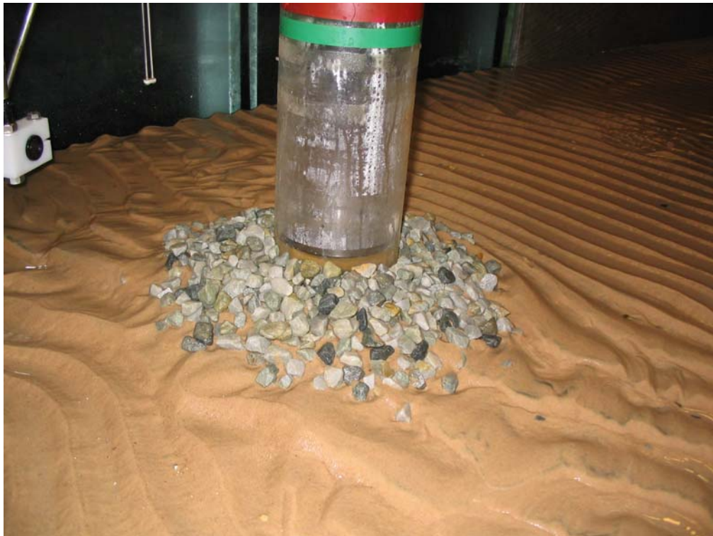
Figure 1.35. Shape of scour protection at the end of 3.5. No severe damage.
