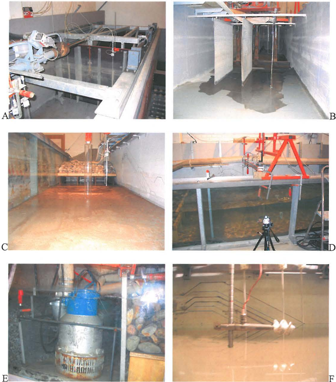
Figure 1.1. A: The paddle. B: Diffuser and guiding walls. C: Model in front of stone beach with a flow tunnel to increase the flow at the bottom. D: Side view with ruler to the left and a video camera in the front. The video footage on the movie DVD is shot through the glass. E: Pump. There are three pumps in all - standing next to each other. F: Propeller for measuring current velocity.
