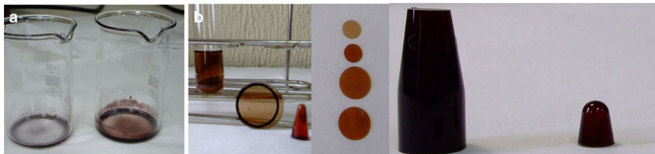
Fig. 4 a Blends of DGEBA and alkyl-coated Au NPs (0.1 wt%) without ( left ) and with ( right ) 3 wt% of amphiphilic polymer; b nanocomposites prepared with 3 wt% of the amphiphilic polymer and 0.1 wt% gold NPs: The test tube shows the aspect of a dispersion of gold NPs in THF
