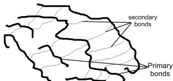
Figure 5. Representation of primary and secondary bonds in a polymeric matrix.
