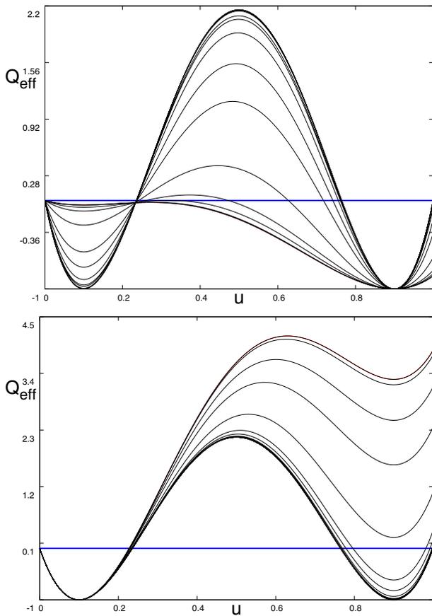
**Fig. 12.**  $Q_{\text{eff}}$  vs.  $u$  for different values of  $\lambda$ . The more asymmetric curve corresponds to  $\lambda = 0$ , then the curves are increasingly asymmetric with  $\lambda$  increasing. (Top)  $\alpha_0 = 0.3$ . (Bottom)  $\alpha_0 = 0.7$ . Values of others parameters:  $\beta b = 0.1$  and  $b_0 = 0.9$ .
