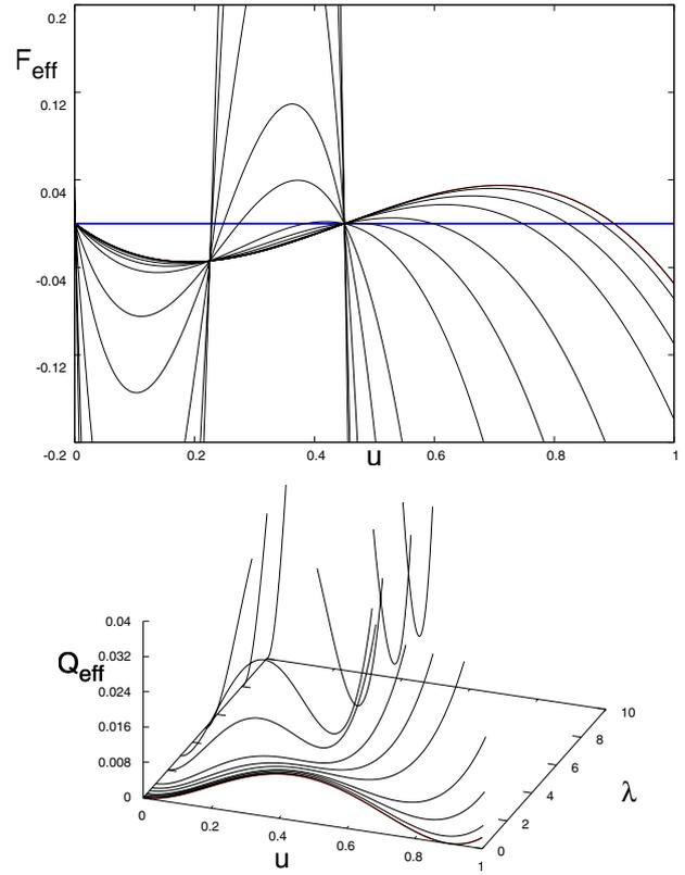
**Fig. 9.** (Top)  $F_{\text{eff}}^{b_0}$  vs.  $u$  for different values of  $\lambda$ . (Bottom)  $Q_{\text{eff}}$  vs.  $u$  for different values of  $\lambda$ .  $\alpha = 0.5$ ,  $\beta b = 0.001$  and  $b_0 = 0.9$ .
