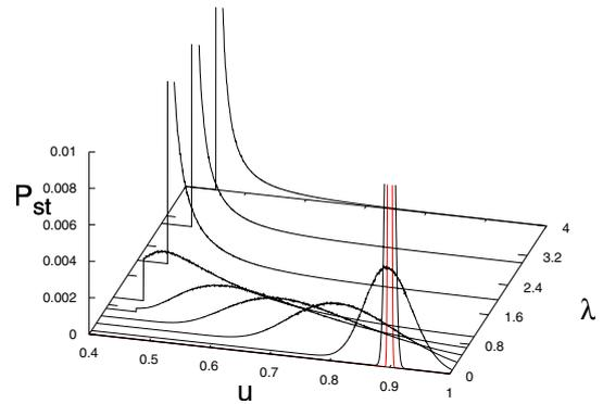
**Fig. 10.** SPDF vs.  $u$  and  $\lambda$  (for  $b$  parameter fluctuations) calculated by simulation of stochastic process ( $P_{st}$ ) by introducing a form which is non-zero uniform over the corresponding basin around the affected solution and the in rest zero, as initial condition.  $\alpha = 0.5$ ,  $\beta b = 0.001$  and  $b_0 = 0.9$ .
