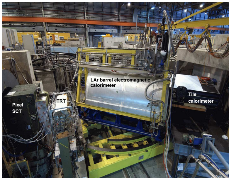
Figure 10.2: Picture of the combined test-beam set-up for the inner detector and the calorimeters. The beam particles come from the left of the picture, traverse the magnet and then hit the calorimeters on the right side of the picture. On the left, just behind the pole tips of the magnet in which the pixel and SCT modules were installed, are the barrel TRT modules. On the yellow rotating support table is the cryostat housing the LAr electromagnetic calorimeter modules and behind it (right side of the picture) are the tile calorimeter barrel (not visible) and extended barrel modules.
