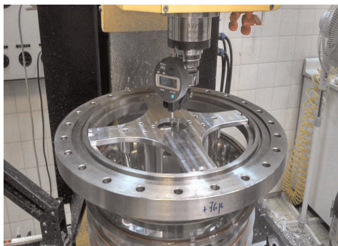
Fig. 2. ESQ's within 100 kV tube during the centering and alignment process.
