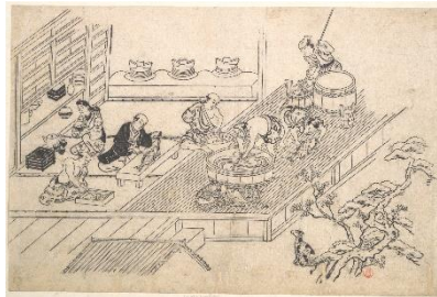
Figures 10: Traditional minka house ground floor entrance area connected with outer environment: lower doma room and kamado kitchen floor surface with elevated tatami living room; [Hishikawa, 1680]
