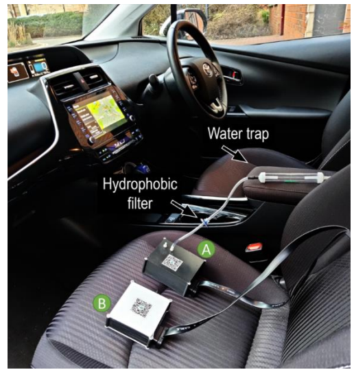
Fig. 6. Physical sensor (A) and digital twin (B) installed inside the vehicle. Labels A and B refer to the same labels as in Fig. 1.
