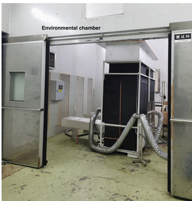
Fig. 4.3. 20 kW cooler unit under preinstallation testing.
