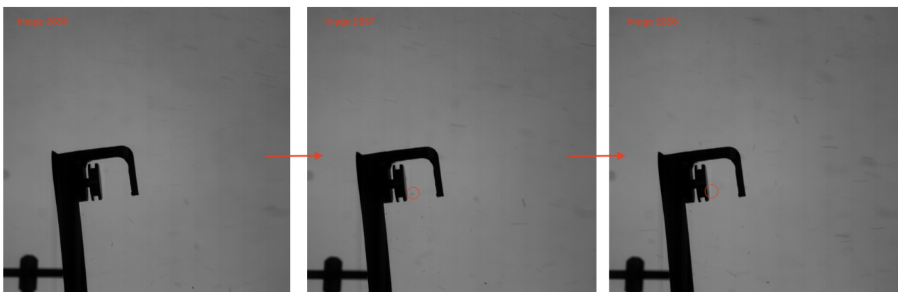
Figure 3.8: These high-speed camera images show a particle hitting the stub within AB1. In the second image a particle can be seen approaching the stub and then sticking to it in the third image. In both cases the particle is highlighted by a red circle.
