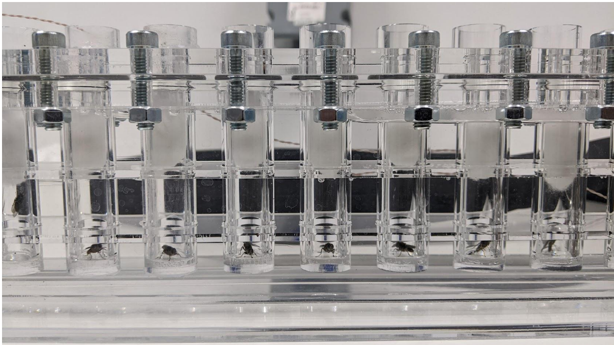
Figure 3.2 Organ pipe set up for CT_{max} experiments. Organ pipes are connected by tubing to Grant LTC4 circulating water baths. Temperature of the inside of the pipes was taken by T type thermocouple. Seen here, G. pallidipes .
