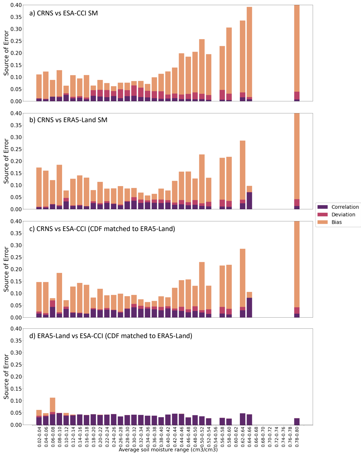
Figure 4.6 shows the influence of rescaling methods on data. 4.6a and 4.6b show the CRNS vs ESA-CCI SM and CRNS vs ERA5-Land SM respectively. The data is the same as in Figure 4.4 although not normalized and the fractional contribution to MSD is projected onto RMSD. Figure 4.6c shows a comparison of CRNS data with ESA-CCI data that has been CDF matched to ERA5-Land data. Figure 4.6d shows a comparison of ERA5-Land SM data and the ESA-CCI data CDF matched with ERA5-Land data.
