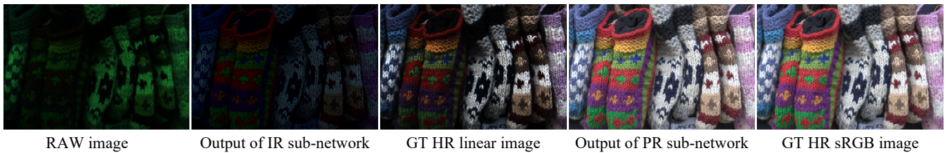
Fig. 13: Visualization of the outputs of two sub-networks ( \times 2 ). The GT HR linear/sRGB images are available in the RAW-sRGB dataset [21]. Images with different resolutions are resized to the same size for displaying. As GT HR linear images are not used in training, the intermediate results generated by IR sub-network have obvious color distortion. However, with the help of ACG generator, false colors can be well corrected by the following PR sub-network.
