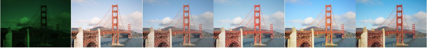
Fig. 2: sRGB images with different camera styles. From left to right: the RAW image, the sRGB images produced by FUJIFILM GFX100S, Nikon D700, Canon 5D Mark II, Sony ILCE-7RM4 and Leica M8. These images are generated by applying Adobe DNG software development kit with different metadata on the RAW image from the MIT-Adobe FiveK dataset [48].
