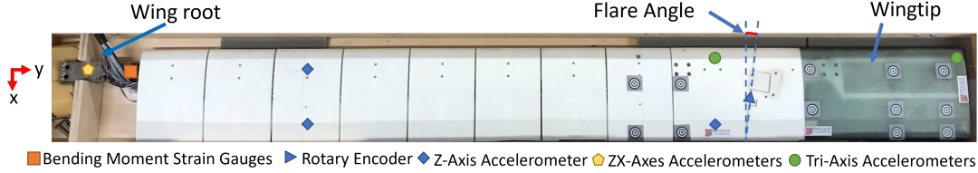
Fig. 4 An overview of the flexible semi-span model Instrumentation
