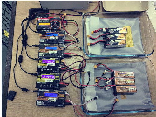
((b)) The battery charging setup with 6 batteries
