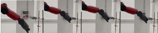
Figure 17. IC1 Experiment: the arm gets “stuck” underneath the bar.
