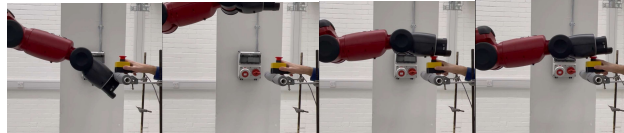
Figure 19. IC3 Experiment: the arm brushes past the bar and is also able to produce the force required to press the button.
