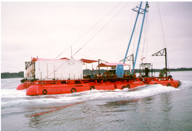
Fig. 38: Geotechnical drilling barge moored over Roca Remolinos in 5 m/s tidal current
