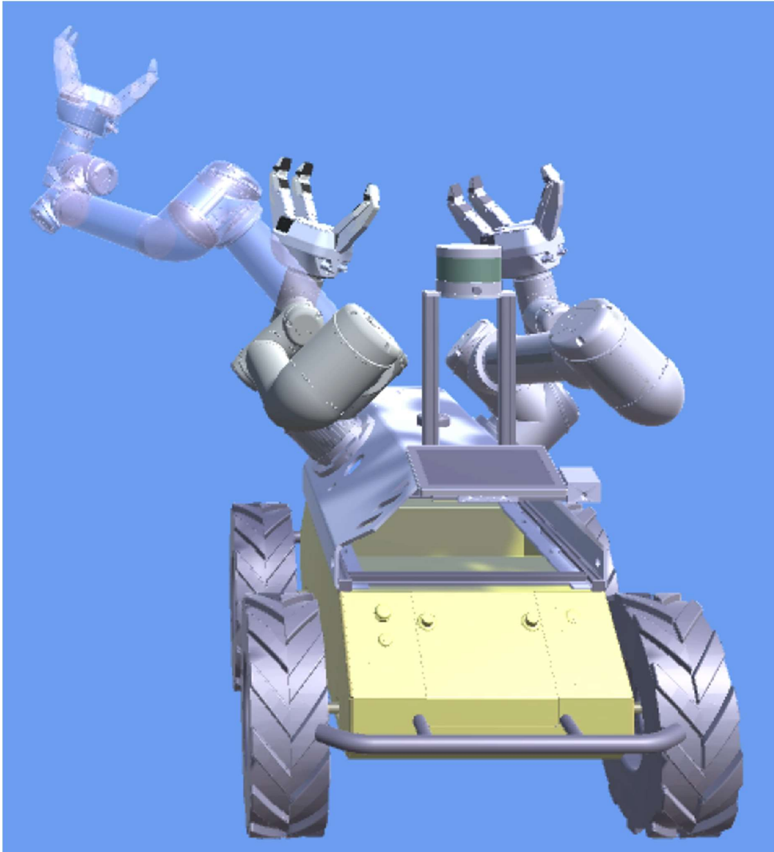
Figure 54: Preview functionality of DT “Ghosting” feature, highlighting the position of the translucent arm, which is the planned movement.
