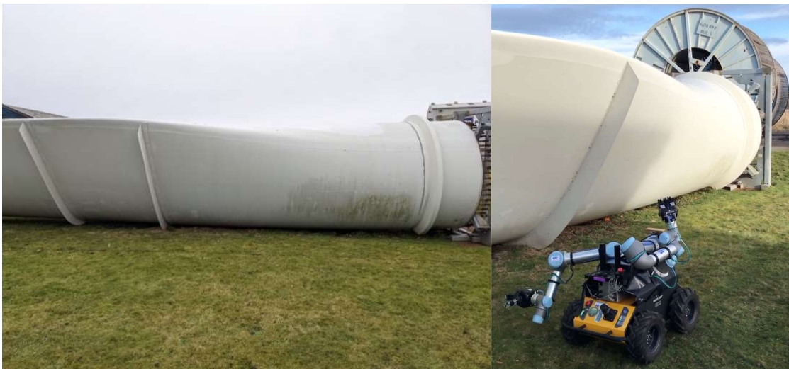
Figure 65: EDF Renewables Hartlepool site visit, showcasing the full blade, the scanned section and the Husky platform performing a scan.
