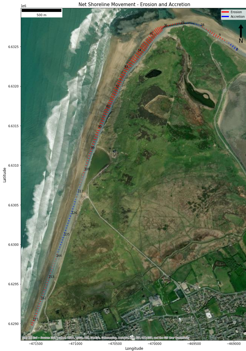
Figure 9: Net Shoreline Movement Erosion and Accretion Output Northam Beach, North Devon. Net Shoreline Movement Output on Saunton Sands, North Devon. Image shows the distance between the oldest and most recent shoreline along each transect. The shoreline change distance of each transect is indicated by a colour gradient shown by the scale bar on the right of the image. Plot coordinates are in WGS 84 / Pseudo-Mercator EPSG:3857 Coordinate Reference System.
