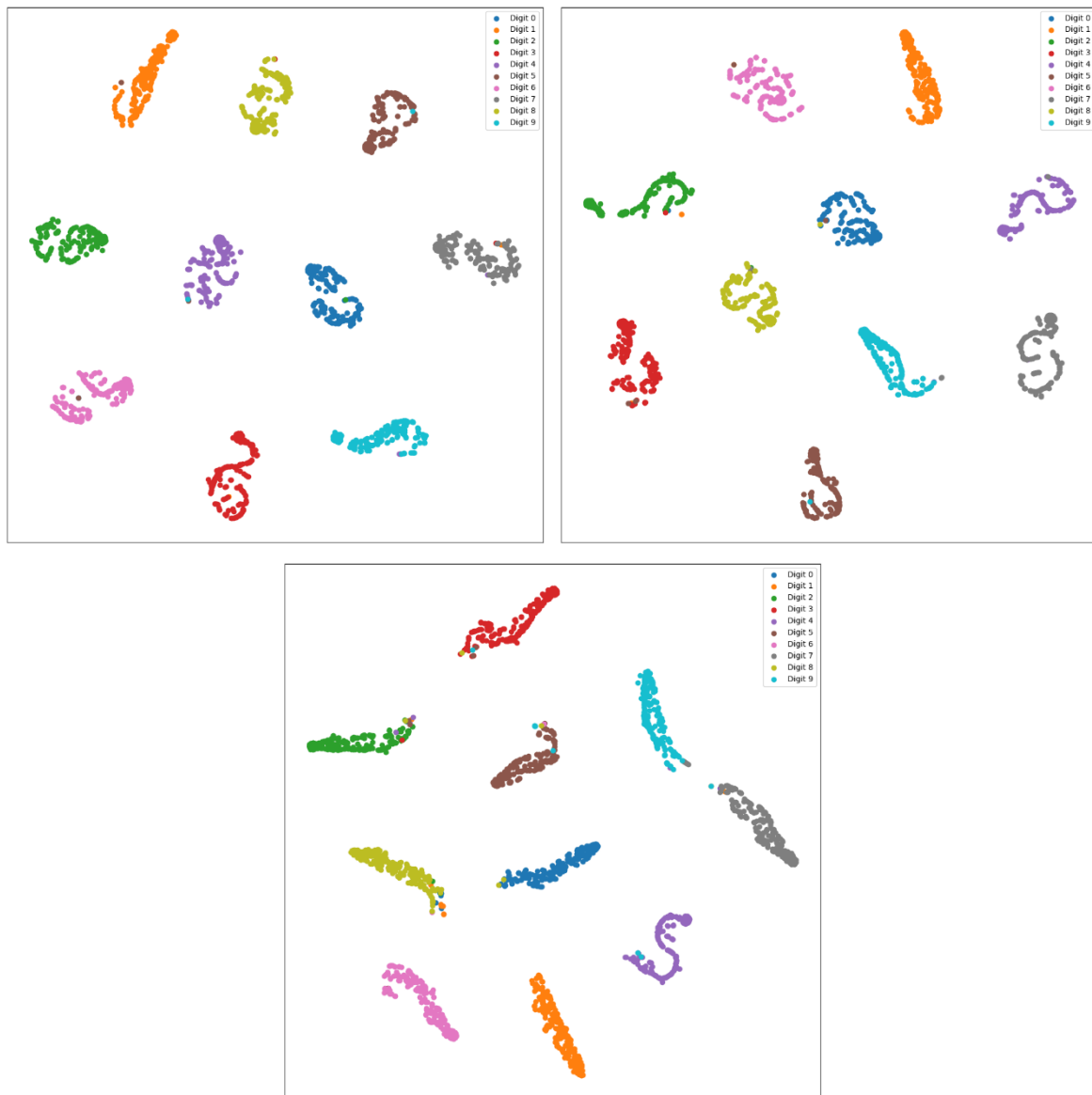
Figure 175:t-SNE plots for the original model (top left) the selected pruned model (97) (top right) an over pruned model (127) (bottom)
