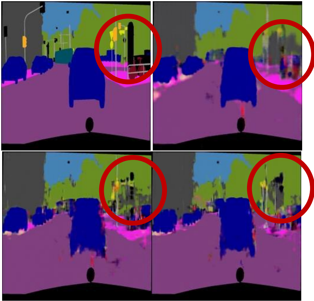
Figure 60: Top left is the ground truth segmentation mask, top right shows the initial trained model before pruning has been applied, bottom left shows the model at pruning step 33, and bottom right shows the model output at pruning step 99.
