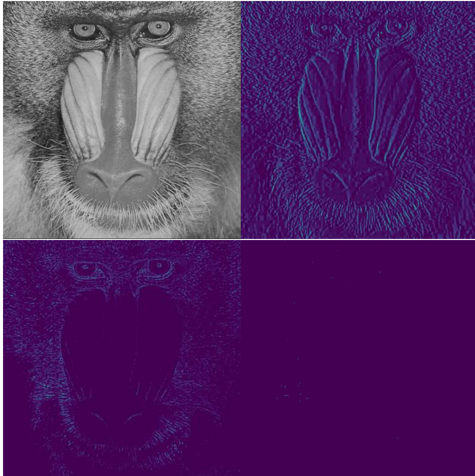
Figure 17: Visualisations of multiple filters from the trained model given one input image. Input image (Top Left) Filter 43 (Top Right – Importance score 0.7) Filter 25 (Bottom Left – Importance Score 0.3) and Filter 30 (Bottom Right – Importance score 0.015) for conv layer 11
