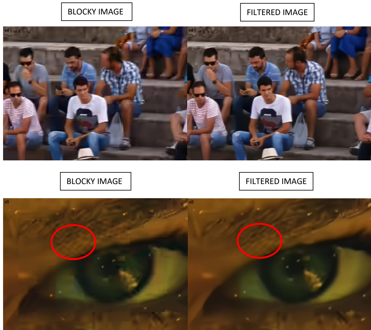
Figure 36: Visual examples of deblocking and smoothing of frames when the machine learning model has been applied.
