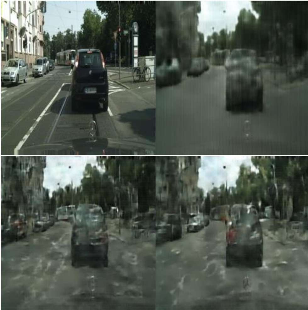
Figure 55: Top left is the ground truth image, top right shows the initial trained model before pruning has been applied, bottom left shows the model at pruning step 33, and bottom right shows the model output at pruning step 99.
