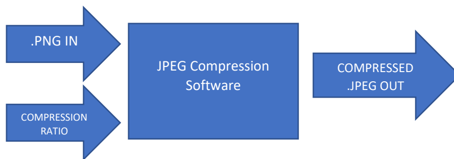
Figure 12: Dataflow in the image augmentation process for compressed JPEG images.
