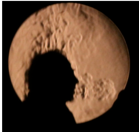
Figure 2. Schlieren photograph of a person talking, showing (i) the cone-shaped turbulent exhalation jet emanating from the mouth and (ii) the vertical thermal plume passing over the face and head.
