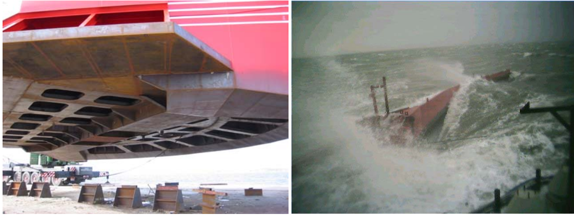
Figure 4. Left: WD prototype at launch in March 2003. The open air-chambers are used to control the floating level. Right: WD prototype in heavy wave conditions.
