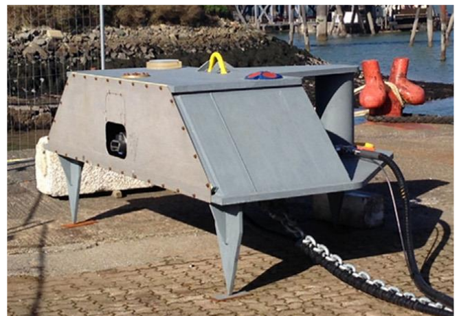
Fig. 4. ADCP in deployment housing from a similar deployment at the same location in Ramsey Sound. Source: [12].
