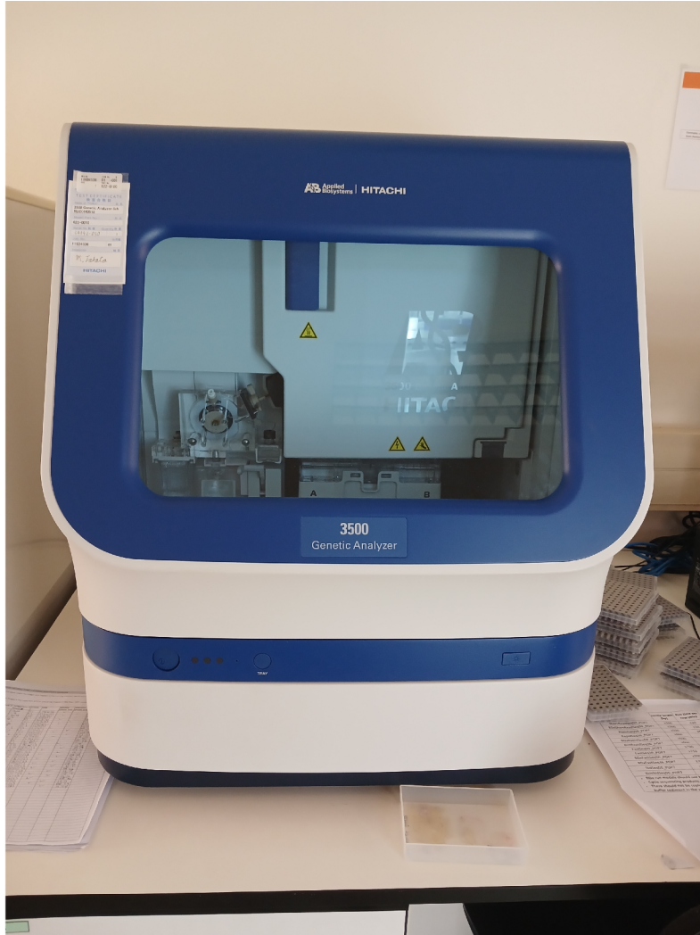
Genetic analyser with plates loaded for capillary electrophoresis.
