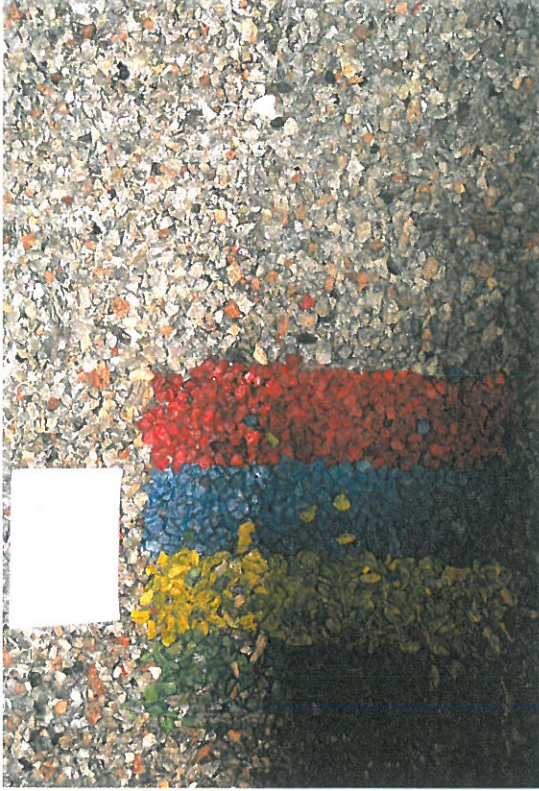
Transport after reshaping: Series 6, H_{m0} = 9,9 cm, T_p = 1,7 sec. N = 400 waves.
