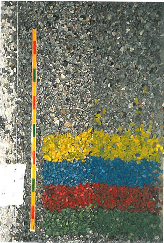
Transport during reshaping: Series 3, H_{m0} = 8,1\text{ cm} , T_p = 1,4\text{ sec} . N = 500, 1000, 2000 and 3000 waves.
