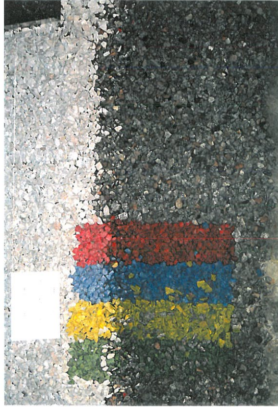
Transport after reshaping: Series 5, H_{m0} = 9,6\text{ cm} , T_p = 1,6\text{ sec} . N = 3000 waves. The red band is now supported and no transport in the red band is showing! Notice, non-coloured stones in the yellow band.
