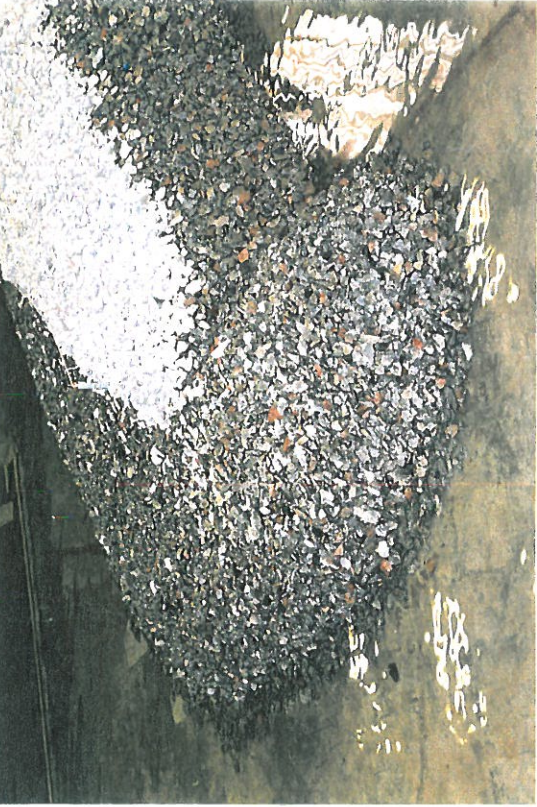
Reshaping of roundhead: Series 6, H_{m0} = 9,5 cm, T_p = 1,7 sec.
