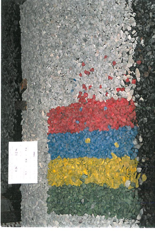
Transport after reshaping: Series 4, H_{m0} = 9,1\text{cm} , T_p = 1,5\text{ sec} . N = 3000 waves. Only transport in the red layer. This is due to the problem concerning the meeting of two different stability-numbers (coloured stones \Rightarrow non-coloured stones).
