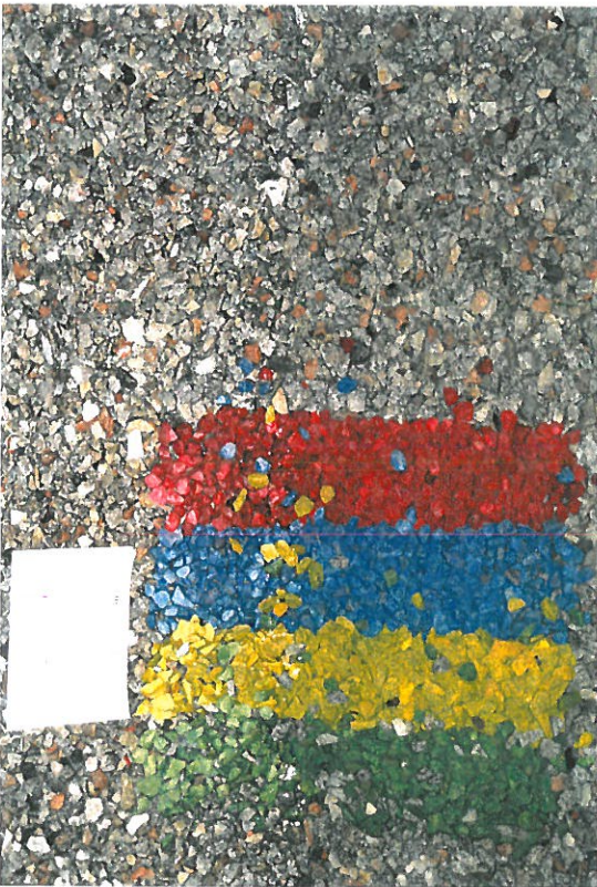
Transport after reshaping: Series 6, H_{m0} = 9,9 cm, T_p = 1,7 sec. N = 600 waves.
