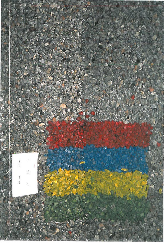
Transport during reshaping: Series 4, H_{m0} = 9,3 \text{ cm} , T_p = 1,5 \text{ sec} . N = 500 and 2000 waves. The red band is still not supported! This causes the red stones to move.
