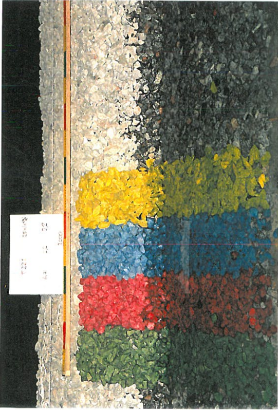
Transport after reshaping: Series 2, H_{m0} = 6,7\text{cm} , T_p = 1,2\text{ sec} . N = 2000 waves. No transport!
