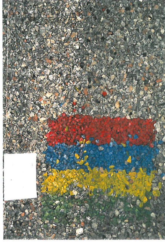
Transport after reshaping: Series 4, H_{m0} = 9,1\text{cm} , T_p = 1,5\text{ sec} . N = 3000 waves. Only transport in the red layer. This is due to the problem concerning the meeting of two different stability-numbers (coloured stones \Rightarrow non-coloured stones).
