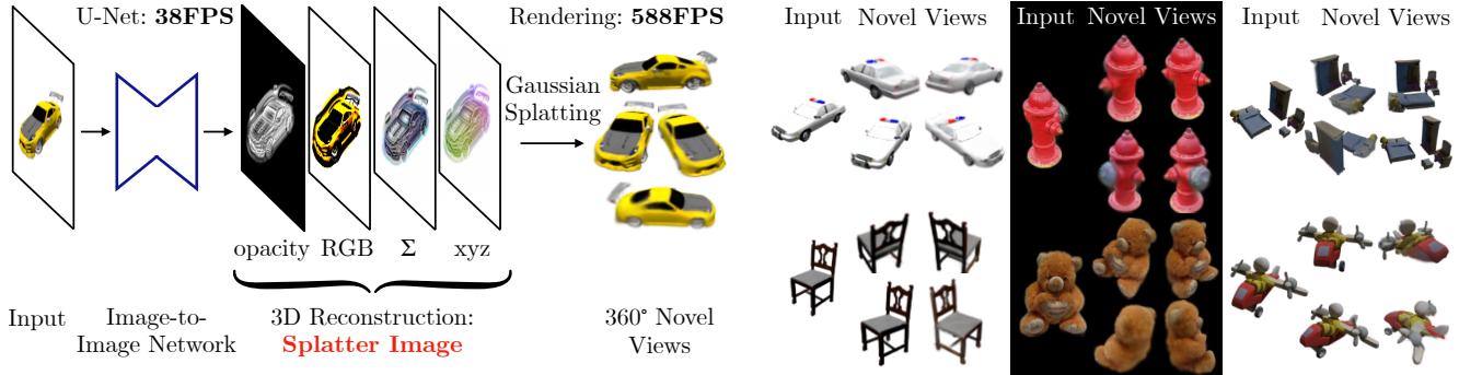
Figure 1. The Splatter Image is an ultra-efficient method for single- and few-view 3D reconstruction. It uses an image-to-image neural network to map the input image to another image that holds the parameters of one coloured 3D Gaussian per pixel. Splatter Image achieves excellent 3D reconstruction quality on synthetic, real and large-scale datasets while using a single GPU for training.
