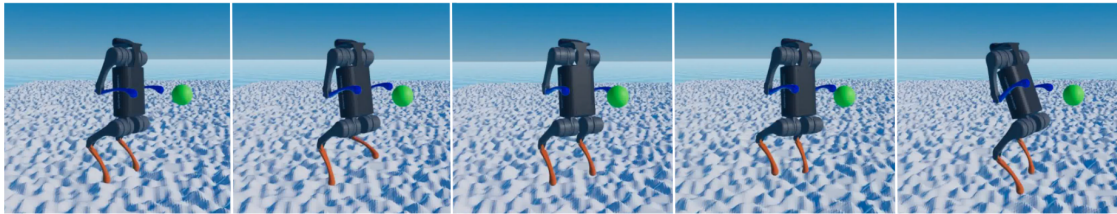
Figure 6.7: The robot was tested on rough terrain to assess the role of the upper limbs in maintaining balance during locomotion.
