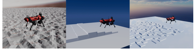
Fig. 4. RaiSim simulation set up for evaluation of blind and perceptive locomotion policies with ANYmal C traversing terrains comprising unstructured ground, stairs and bricks.
