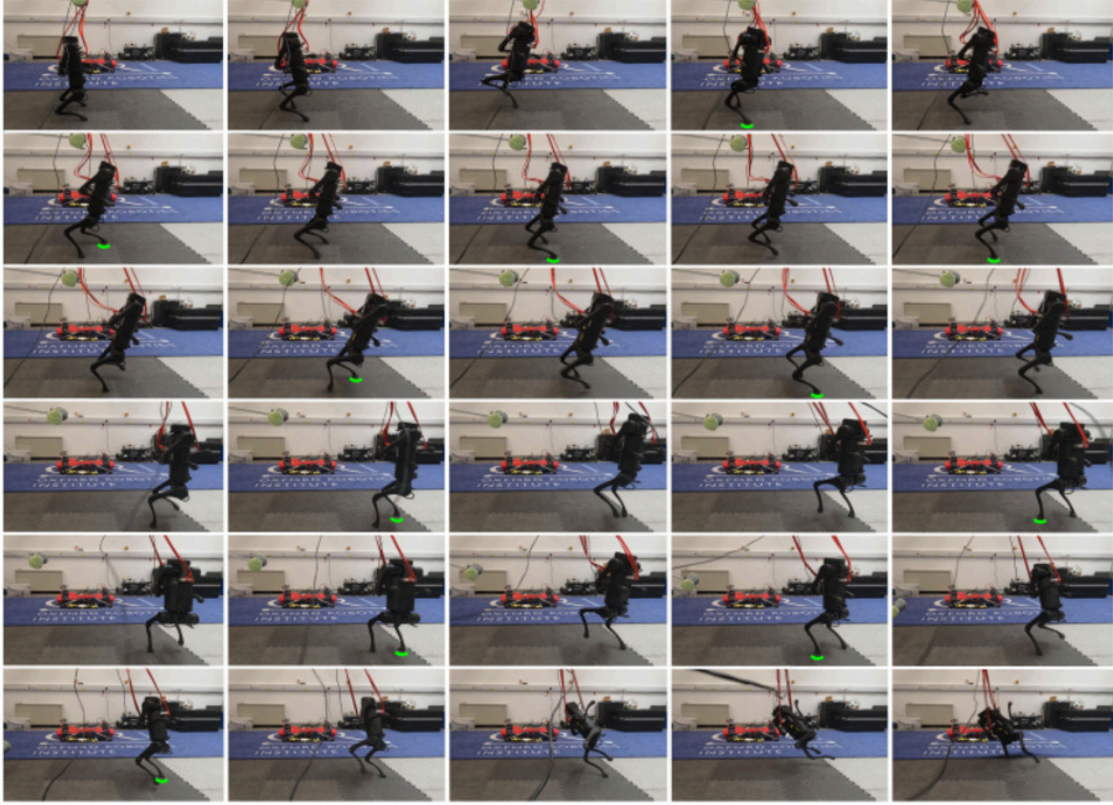
Figure 6.11: Bipedal policy deployed on the Unitree A1 robot, the green lines underneath the feet indicate the steps taken. Note that the slings are kept loose during the whole experiment.
