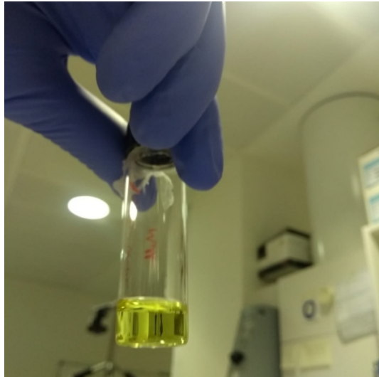
7.3 DFHBI partitioning into oil phase. Intense discoloration of a mixture of 1:1 Hx:Si incubated with 60 \mu M DFHBI.
